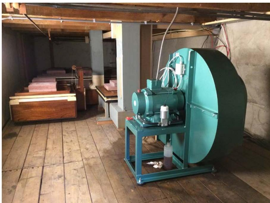
**A brand new, high capacity organ blower underneath the floor, blowing into three bellows. On the left side bellows a regulation box and string is visible.**
