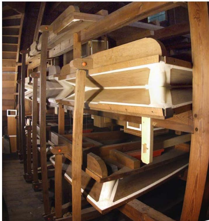
**Inside the bellows chamber an equal amount of 8 huge bellows were situated in a smart configuration.**
