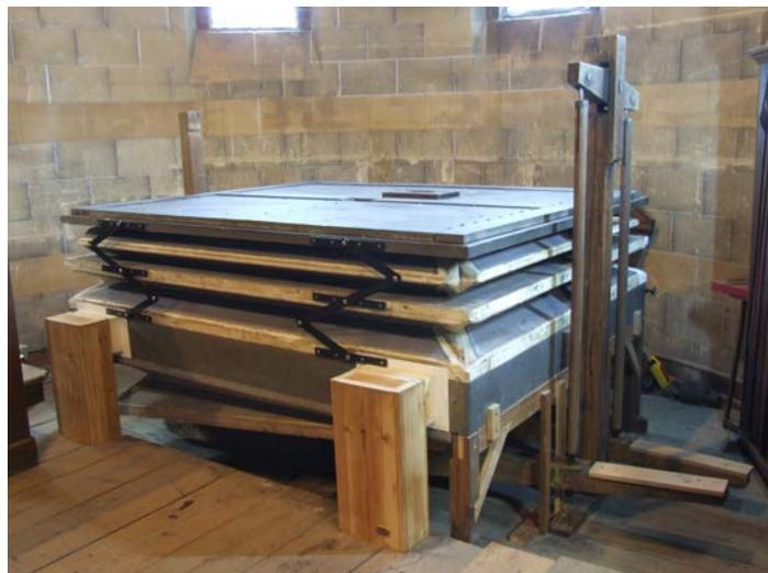
**During the winter of 2019, we consolidated and partly restored a complete reservoir with bellows unit, originally produced in 1895. This unit is situated freely on the organ balcony. This makes it easy to see how everything works. Behind the reservoir the blower still does its work, but everything is as it was again.**
