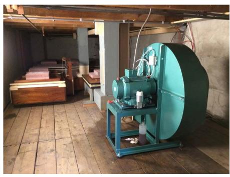
A brand new, high capacity organ blower underneath the floor, blowing into three bellows. On the left side bellows a regulation box and string is visible.
