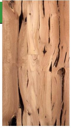
Longitudinal surface of a glued up Lavandula angustifolia wood specimen, containing both flat sawn and quarter sawn wood
