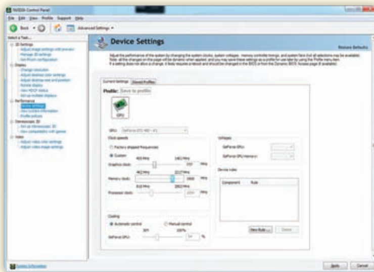
Adjusting clock speeds for the graphics card under the Nvidia Control Panel
