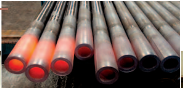
Upsetted extremities of Drill Pipes
