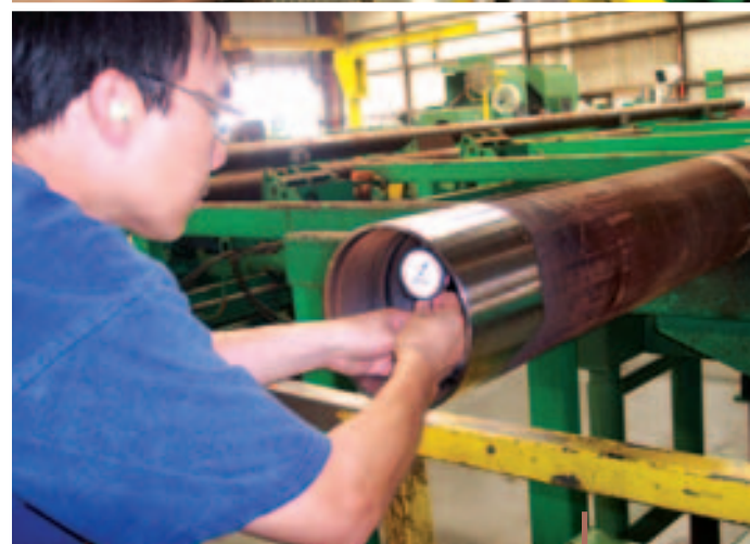
Inspection VAM® SLIJ-II box end
