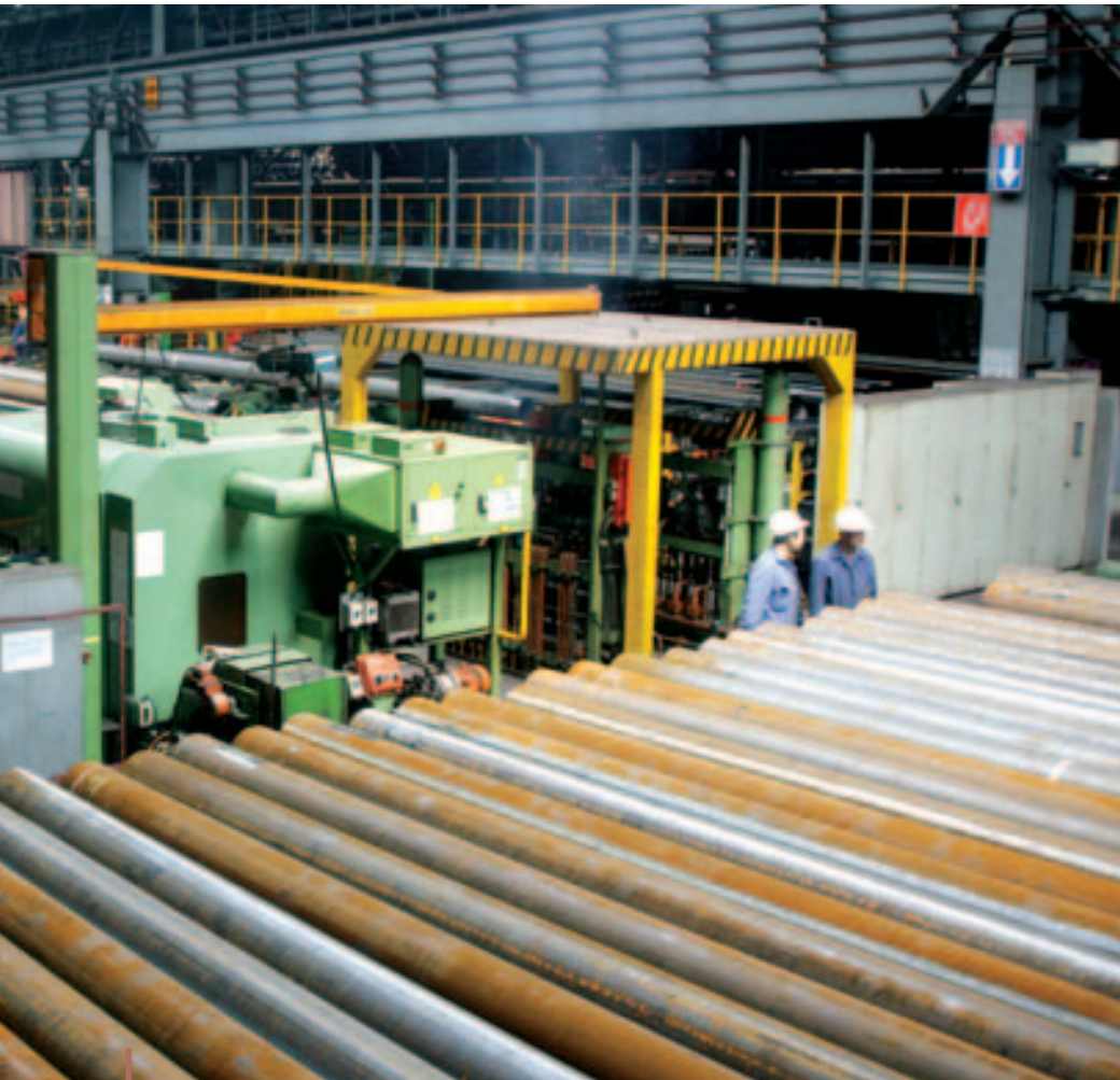
The production line for casing threads also cuts state-of-the-art riser pipes to customer requirements
