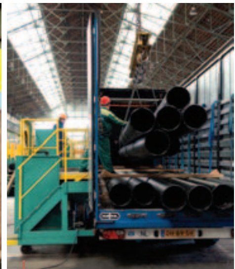
The criteria for loading trucks doesn't only guarantee the quality of the pipes throughout the way, but above all takes into account the safety of all personnel concerned
