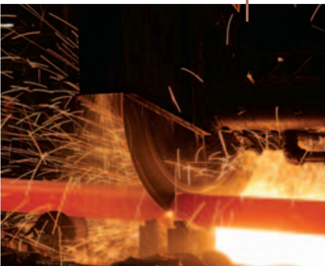
Hot saw cutting pipe to specified length
