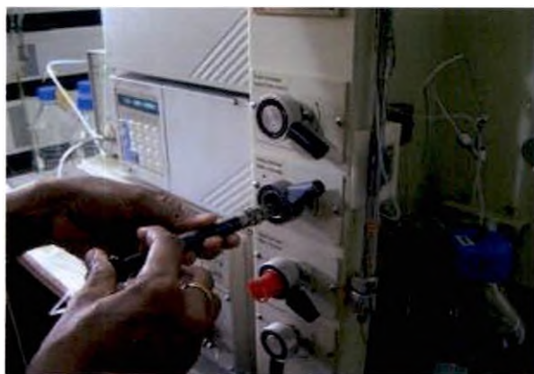
Plate 6b. Injection of the prepared seed extract sample of Strychnos nux-vomica into the High Performance Liquid Chromatograph
