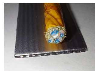
Figure 4. FFC cable versus standard SpW cables
