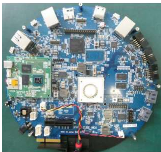
Fig. 3. The outlook of Space Cube ® mk4 and its interior assembly
