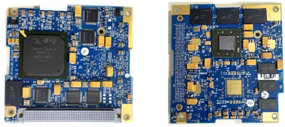
Fig. 6. NuStream board: Front side (left) carries RC64. The FPGA is shown on the back side (right).
