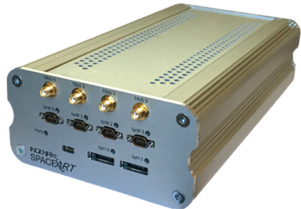
Fig. 5. SpaceART SpW Sniffer hardware unit.
