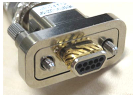
Figure 8. Example of EMI clip integrated in a MD9 male connector
