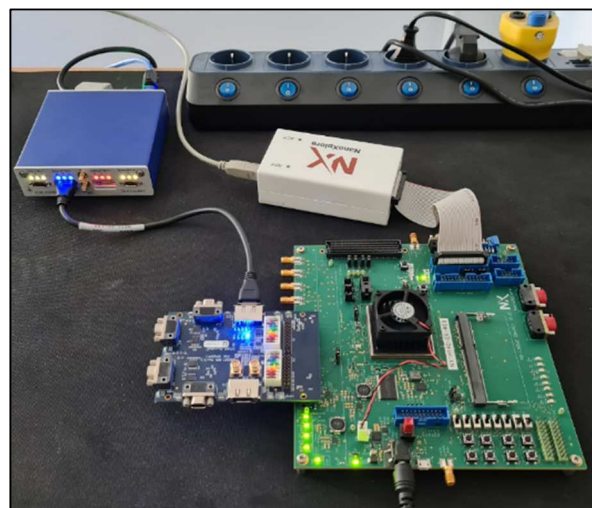
Fig. 1. BRAVE SpFi Interoperability Test with a STAR-Fire Mk3 unit.
