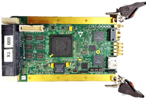
Fig. 5. VPX64 board (3U-VPX form factor) showing RC64. Boot flash is mounted on the back side of the board. No Host is used.
