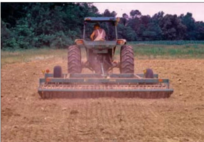
Fig. 5.30 When top-sowing nwsg on a seedbed prepared by conventional tillage, cultipacking ensures firm seed-to-soil contact and improves germination rate and initial growth. Top-sown seed should not be covered by disking.
