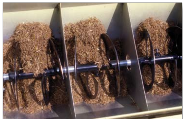
Fig. 5.23 and 5.24 Drills with “picker wheels” and agitators in the seed box (such as this Truax™) are recommended when planting bluestems and indiagrass. This ensures an even flow of seed and prevents seed lodging in the box.
