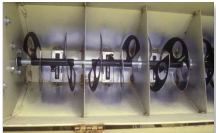
Fig. 5.23 and 5.24 Drills with “picker wheels” and agitators in the seed box (such as this Truax™) are recommended when planting bluestems and indiagrass. This ensures an even flow of seed and prevents seed lodging in the box.
