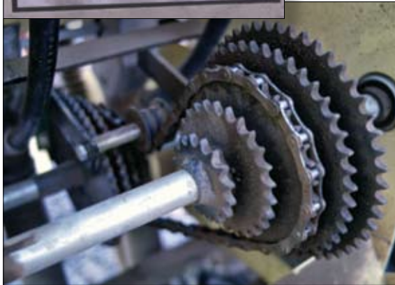
Fig. 5.26 Seed output is adjusted on some drills, such as this Truax™, by a chain sprocket.
