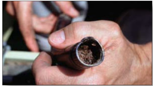
Fig. 5.27 It is critical to check drills thoroughly before use. Not only must the drill be calibrated before planting (according to PLS estimation), but general maintenance is also required. This drill wasn't planting switchgrass. Why? The drop tubes coming out of the small seed box were clogged. Drop tubes, chain sprockets, seed boxes and grease fittings all need attention before planting.
