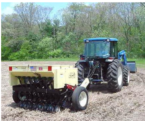
Figure 6. A no-till drill, such as a Truax® (pictured) or Great Plains® seeder, is the most effective means to plant fluffy warm-season grass seed. Photo by Paul Rothbart.
