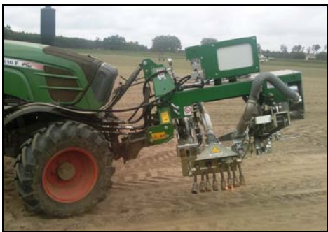
Fig. 3: Side view of the front-mounted flamer
