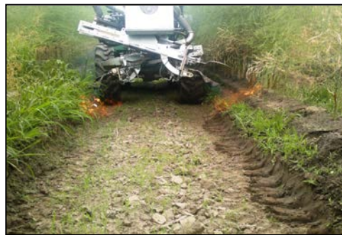
Fig. 4: Double boom intra-row flamer at work
