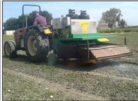
Fig. 2: Broadcast flaming in the harvest phase
