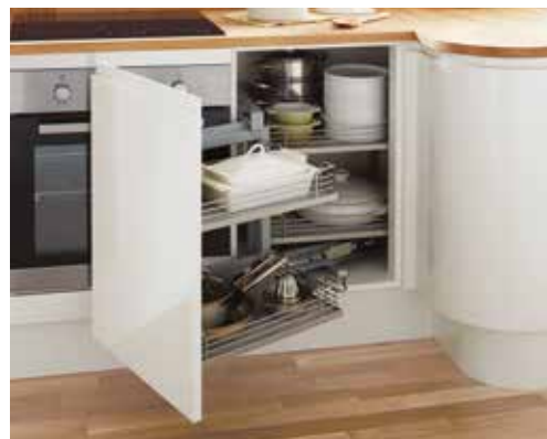
Corner storage accessory* 1000mm wide left hand 1000mm wide right hand 0.138m 2 storage space per front basket 0.159m 2 storage space per back basket 7kg maximum weight per front basket 9kg maximum weight per rear basket 4 large storage baskets with anti-slip coating and solid base; can be used in corner base or tower corner larder units
