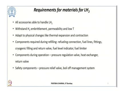
Now, there are materials requirement when we talk about liquid hydrogen storage. The important requirement is that all the accessories, the storage tank, the peripheral equipments, components, all needs to be able to withstand that temperature of the liquid hydrogen. So, they should be able to handle that liquid hydrogen temperature.
