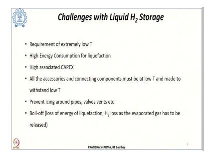
Now, the problems which are there when it comes to storing liquid hydrogen is we know that this hydrogen has to be stored at 20 K which is a very low temperature. We have already seen that it involves very high energy consumption when we liquefy it. At the same time the cost associated with liquefaction is also very high.
