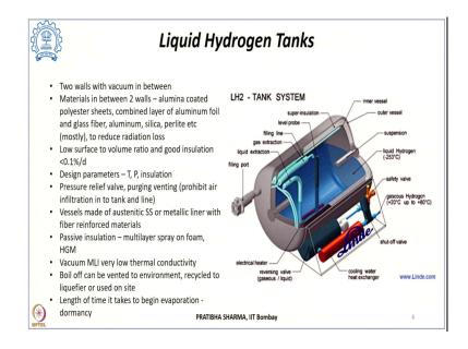
Now, if we see the design of a liquid hydrogen tank, it is basically made up of two tanks or it is two walls in the tank. So, an outer wall and an inner wall and in between is the vacuum in such tanks. So, these are super insulated vessels. There are two walls with vacuum in between.
