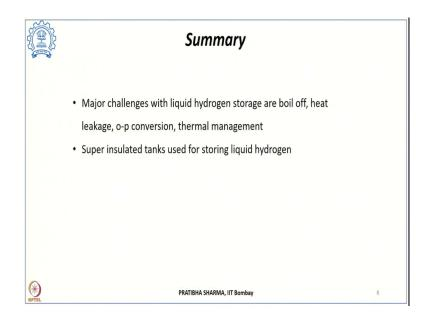
To summarize this part, we have seen in the various liquid hydrogen storage systems, what are the major challenges associated with that. The major challenge being like boil-off, if there is any heat input, or the incomplete ortho to para conversion that can also lead to an exothermic reaction.
