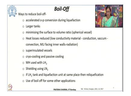
So, we can we have to consider the ways in which we can reduce this boil-off which is the major challenge when storing hydrogen in the liquid state. So, there can be ways in which we can reduce that. During liquefaction we have to convert it into parahydrogen. So, the equilibrium composition should be 99.8 percent of parahydrogen at the liquefaction temperature. So, it should be an accelerated ortho to para conversion which needs to be done during liquefaction.
