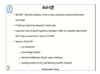
Now, this boil-off is in fact, correlated with the thermal insulation, how well is the tank insulated, because we have to stop any heat inflow from the surroundings into the storage vessel. The reason is we are storing hydrogen at 20 K and there is a very large temperature difference between the ambient and the temperature at which we store. So, we have to use very good thermal insulation, so as to prevent any heat inflow into the storage system.
