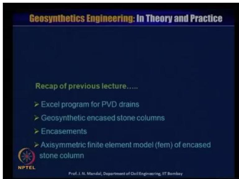
I will now address recap of previous lecture is Excel program for prefabricated vertical drain, geosynthetics encased stone columns, encasements, and Axisymmetric finite element model F E M of encased stone column.
