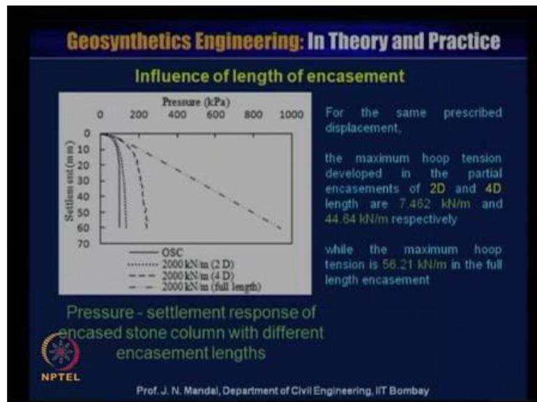
Now, what are the influences of the length of the encasement, now here show that pressure settlement response of encased stone column with different encasement length. So, this means that we know that what will be the diameter of the stone column, so length will be, we have taken 2 D length we have taken 4 D length and we have taken 5
