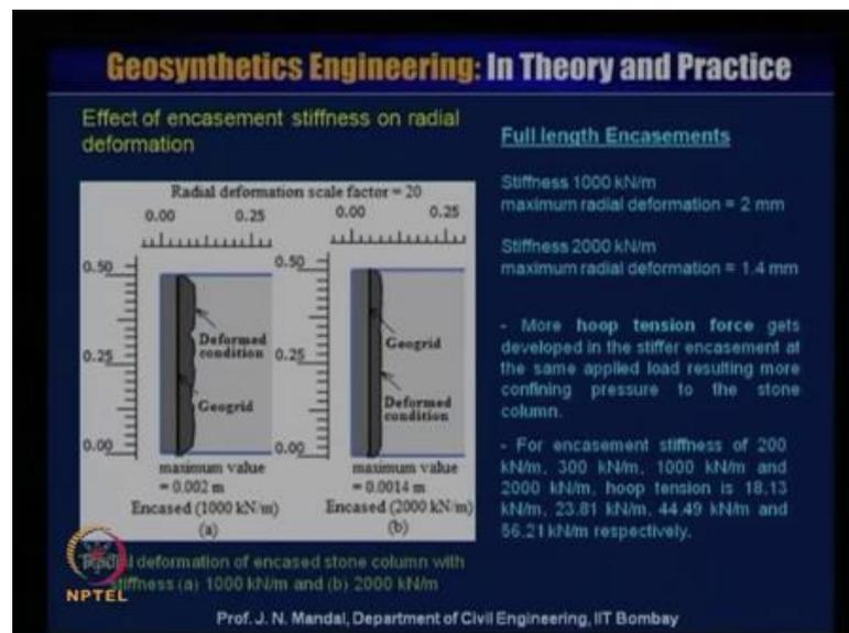
Now, effect of encasement stiffness on radial deformation, so here this figure show that radial deformation of encased stone column with the stiffness 1000 kilo Newton per meter this a and for b this stiffness is 2000 kilo Newton per meter. You can see here that
