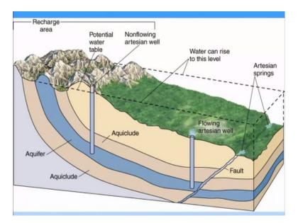
So, this is the same diagram, which you can go through, which talks about the different groundwater bodies, aquifer, aquiclude, artesian well, artesian spring, etc.
