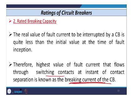
So, the real value of current that is to be interrupted by breaker that is lower than the actual value at the time of fault. So, therefore, the highest value of fault current that flows through the switching contacts or the contacts of the circuit breaker at the instant of contact separation that is known as the breaking current of Circuit Breaker.
