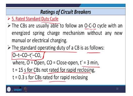
So, if I just want to define, this Standard Duty Cycle, then this breaker that should allow the opening closing and opening operation of the cycle within certain period of time. So, if I just want to define the standard operating duty of the Circuit Breaker then that is given by this equation.
