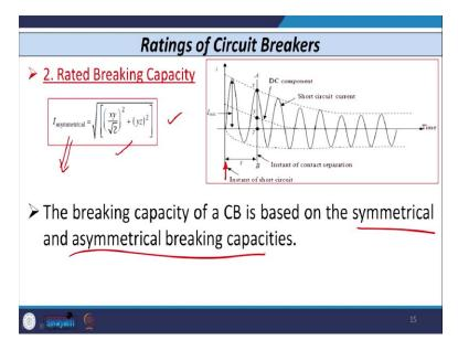
We can say that it is I asymmetrical breaking current that is defined as by this equation X Y by root 2 whole square plus Y Z whole square, so, X and Y points are here and Y is here and Z point is here. So, you can find out the Asymmetrical Breaking Current. So, the breaking capacity of Circuit Breaker that is based on the symmetrical as well as asymmetrical capacity of the Circuit Breaker.
