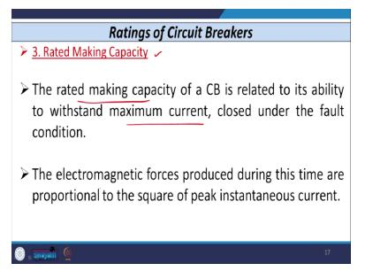
Now, let us discuss what is the Rated Making Capacity. Now as I told you breaking capacity of Circuit Breaker that comes or that is defined whenever the contact of the Circuit Breaker that becomes open or separate. The Making Capacity of Circuit Breaker comes in picture when the contact of the Circuit Breaker closes.
