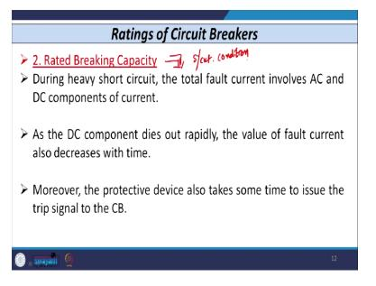
Okay, so, the second point that is known as Breaking Capacity or the Rated Breaking Capacity of the Circuit Breaker. Now, this definition that comes picture again under the short circuit condition. So, we know that during heavy short circuit, the total fault current that involves the transient component that is the decaying DC component as well as the steady state component all were known as DC component.
