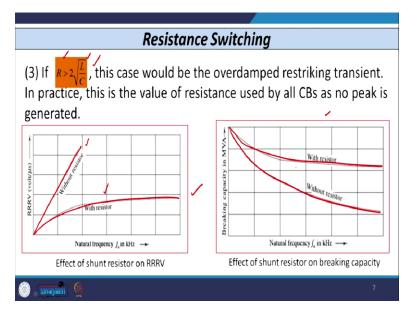
And the third case if I assume, R is greater than the 2 under root LC, then this case that would be overdamped restriking case and this type of value that is R, the value of R is greater than this value that is actually used in practice, because in this case the no peak is generated as it was generated in earlier 2 cases. So, again, these whenever the steady state value that is established or achieved that is achieved without any peak.
