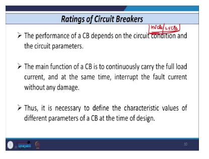
So, with this background let us first discuss, what is the rating of Circuit Breaker. So, this we will discuss about the High Voltage Circuit Breakers. However, it can be also applicable to Low Voltage Circuit Breakers also maybe the definition that may change slightly, in case of Low Voltage Circuit Breakers.
