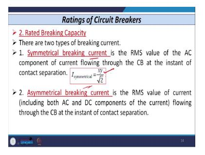
So, now the there are two types of breaking current: one is known as Symmetrical Breaking Current and the other is known is Asymmetrical Breaking Current. So, the Symmetrical Breaking Current that is defined as the RMS value of AC component of current that is flowing through the Circuit Breaker at the instant of contact separation. So, that is known as the Asymmetrical Breaking Current and it is defined by I symmetrical that is equal to some points on the graph divided by root 2.
