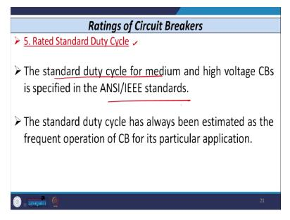
The fifth one that is known as the Rated Standard Duty Cycle of the Circuit Breaker. So, the standard duty cycle of the circuit breaker may be for medium or high voltage circuit breaker that is specified by IEEE or ANSI standards. And this standard duty cycle has always estimated based on the maybe what type of function they need to perform by the breaker.
