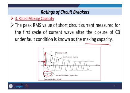
So, this peak of the making capacity that is given by the term root 2 that is the peak value with some constant into the symmetrical breaking capacity of the breaker. This we have already defined, where this constant that is the maximum asymmetry that exists in the fault current wave shape and its value that is usually 1.5 to 2. So, here I have considered 1.8.
