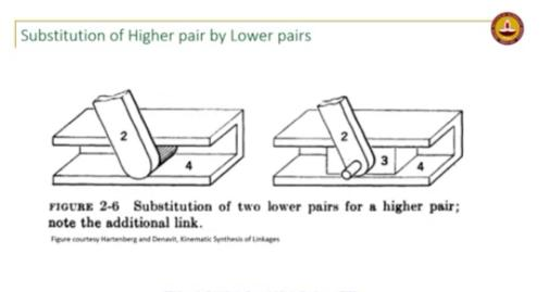
TK Center for Rehabilitation Research & Device Development (R202) https://home.itm.ac.inir2d2 so in this case you have a link, this link to has a pin attached to it which kind of rolls and slides in this slot, okay.
