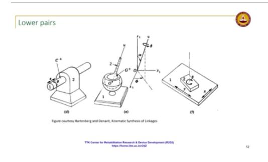
more lower pairs you have in this case unlike the screw joint you have what is known as a cylindrical pair, and here the two motions are independent, you can have rotation which is independent of the translation, okay, so that in the case of the screw that was not the case, the rotation was dependent on the translation or vice-versa.
