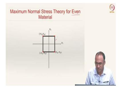
Let us now compare all the theories that we have discussed for brittle materials. The failure of brittle materials can also be represented by maximum normal stress theory which is also sometimes used. For an even material  $\sigma_{ut} = \sigma_{uc}$ . Hence, it is a square and is symmetric about the  $\sigma_1 - \sigma_3$  plane; that is the failure surface for maximum normal stress theory of an even material.
