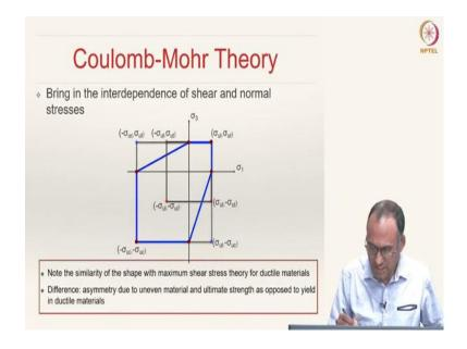
The Coulomb-Mohr theory brings in the interdependence of shear and normal stresses. And please note the similarity of the shape with maximum shear stress theory for ductile materials. The only difference is that asymmetry due to uneven material and ultimate strength as opposite to yield in ductile materials.
