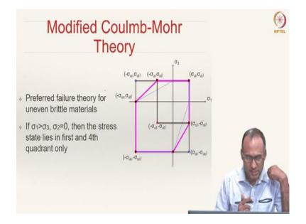
The Modified Coulomb-Mohr Theory is the most preferred failure theory for uneven brittle materials and if  $\sigma_1 > \sigma_3$  and  $\sigma_2 = 0$ , then the stress-state lies in first and fourth quadrant only.
