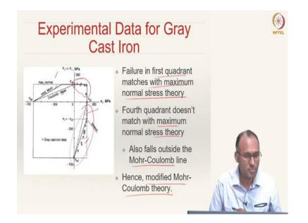
Here, we are seeing experimental data for gray cast iron plotted on all the four theories; actually 4 theories that we have shown in the previous slide, right? Here, you have maximum normal stress theory (uneven materials), Coulomb-Mohr theory and modified Mohr-Coulomb theory. The solid lines are modified Mohr-Coulomb theory. Note that, in
