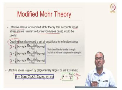
In the case of ductile failure, we have a very nice way of calculating factor of safety; what was that? Irrespective of the complexity of the stress-state may be, we have been calculating something called equivalent stress or von-Mises stress.
