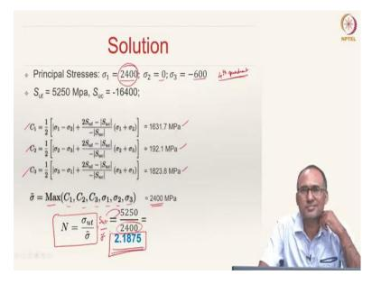
The principal stresses turn out to be 2400 MPa, 0 MPa, -600 MPa; that means, this is in the fourth quadrant. If you are in the first quadrant, you actually do not need to do such a complicated calculation because in the first quadrant your maximum normal stress theory itself will work.
