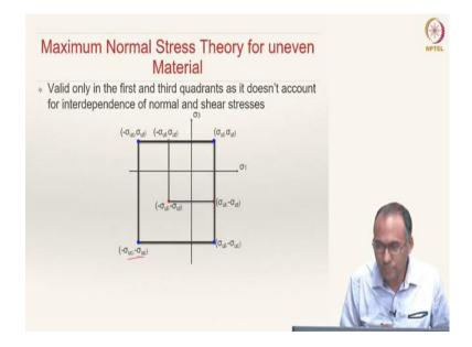
For an uneven material  $\sigma_{ut} \neq \sigma_{uc}$ . The inner square is for even material and the outer square is for uneven material because only on the compressive side your strength is changing tensile strength is the same. So, please note that this theory is valid only in the first and third quadrants as it does not account for interdependence of normal and shear stresses.
