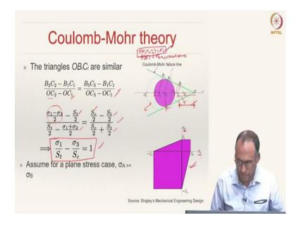
Let us now look at this failure theory; how do we go about prescribing this failure theory. We need to write a functional form to describe the failure theory. In the very beginning, we have said any failure theory can be expressed as
