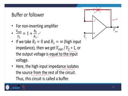
So, here what is done is that your output is shortened to the inverting input terminal over here as you can see in this figure. So, this is short end, this feedback now this is directly connected to this one that is the inverting terminal. So, for the non-inverting amplifier, we have seen,
