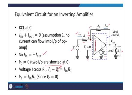
So, let us look at the equivalent circuit for an inverting amplifier. So, here as we assumed that this is, we shorted it here the signal is provided from the inverting terminal and the non-inverting terminal is earth grounded. So, this is the ideal model you have some load over here, you get the output voltage over here and this is the output current that is supplied through the feedback and you have the input current over here.
