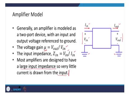
Now, let us look at and try to understand the model of the amplifier. So, generally, an amplifier is modeled as a two-port device with the input and the output voltage reference
