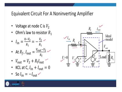
Now, let us look at equivalent circuit in order to analyze this thing. So, if we look at the equivalent circuit over here. Again this is the input voltage this I have grounded. So, this is 0, this is my input current, this is my output current and these two terminals are shortened with the assumption which we have taken.
