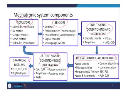
This block diagram essentially shows the important mechatronics components. Where you can see that usually, an actuator and there is a sensor and you have an input signal conditioning and interfacing. Then you have the digital control architecture and output signal conditioning and interfacing and then we have a display for viewing purposes.
