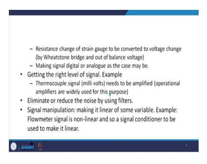
And making signal digital or analog as the case may be then getting the right level of the signal. As I said the thermocouple signals are very minute in the range of millivolt. So, we need this signal to be amplified, and as we are going to talk in the coming slides about the operational amplifiers. These operational amplifiers are widely used for the amplifying purpose of these signals.
