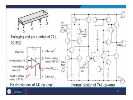
This is how it looks like as I said dual pins are there. You have the two lines of the pins, here 1 2 3 and this is 4, 5, 6, 7, 8. So, there are eight pins in it and this is packaging and pin numbering of 741 op-amp amplifier and there is a mark here just to identify that from the left-hand side of that you have to start counting the pins.
