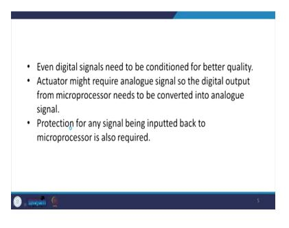
So, the digital output from the microprocessor needs to be converted into the analog signal, for example, if you take the case of a DC motor control. So, you need to give the DC motor an analog signal, and the signal coming out from the microprocessor they are digital in nature.
