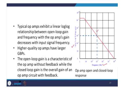
So, this is the typical op characteristic if we plot frequency versus open loop voltage gain. So, this is the curve which you are going to get op-amp and closed loop response, this is what we are going to get. So, the typical op-amp exhibits a linear log relationship between the open-loop gain and the frequency with the op-amp gain decreasing with the input signal of frequency.
