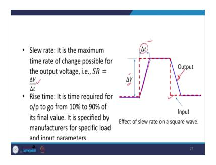
So, this is how the slew rate is defined. So, this is the input the red color is indicating the input and the blue color is indicating the output. So, you can see that the output is not same as that of the input. So, this is your output. So, how much time this deviation is at, how much time it is going to peak this input voltage,e and what is this  $\Delta V$ ?
