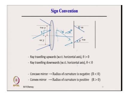
The sign convention is shown here. If the ray as I already mentioned, so, this is a lens which is shown for example. A ray which is incident in the lower half, so, this is the position of the ray will have a negative displacement. So, the displacement is considered or measured from the axis of the system.
