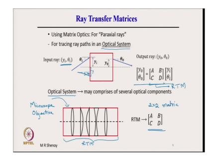
So, the ray transfer matrices we have to determine the ray transfer matrices of an optical system. An optical system here we refer to it shown as a black box here. So, you have an optical system which may comprise of many many optical component for example, the optical system here shown may comprise of several optical components.
