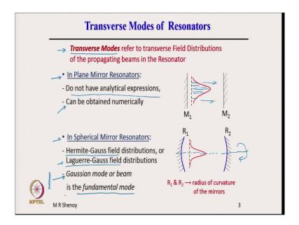
Further the transverse modes of a resonator. We will discuss this transverse modes in detail, but right now transverse modes refer to transverse field distributions. We have seen so far longitudinal modes, which are the resonance frequencies, which are determined by the length of the resonate.
