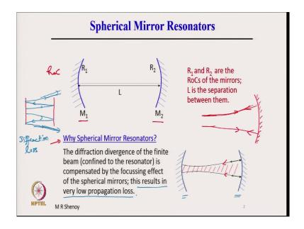
A spherical mirror resonator comprises of two spherical mirrors here M 1 and M 2 are two spherical mirrors of Radius of Curvature RoC, RoC radius of curvature R 1 and R 2 and the mirror separated by a distance L. So, R 1 and R 2 are the RoCs of the mirrors, L is the separation between them.
