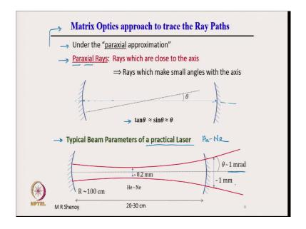
In this part to study the spherical mirror resonators, we will use matrix optics. So, matrix optics approach to trace ray paths. Now, matrix optics is valid under paraxial approximation. What is this paraxial approximation? Now, paraxial rays means rays, so, para-axial. So, it is close to the axis rays which are close to the axis that is the literal meaning of paraxial rays; that means, rays which make small angles with the axis.
