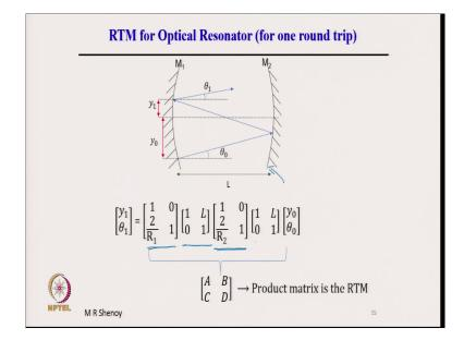
And, therefore, the RTM for the optical resonator for one complete round trip is given here that y 1 theta 1 is equal to. So, we start with y 0, theta 0 this is our starting point y 0 theta 0.
