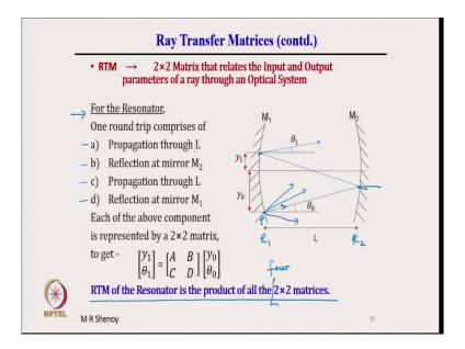
Now, if we consider straight go to the optical resonator our problem is optical resonator not zoom length. So, the optical resonator comprises of two mirrors separated by a distance L. Now, if a ray starts from here, let us say the ray starts from a point P here. It has a displacement initial displacement y 0 and an angle that it makes with the horizontal theta 0. The ray is allowed to go at a particular direction. We can also of course, consider a ray which travels like this.
