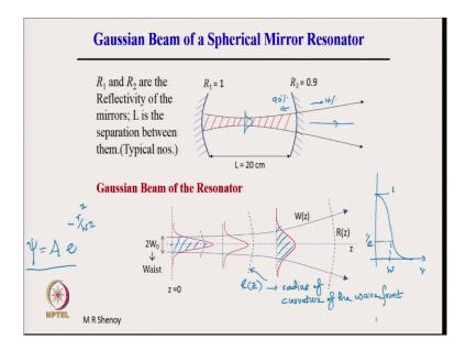
So, these are the two primary reasons why we go for spherical mirror resonators. The Gaussian beam of a spherical mirror resonator is again illustrated here. So, what is shown is a spherical mirror resonator one of the mirrors is assumed 100 percent reflecting which means the reflectivity R 1. So, R 1 here is the reflectivity; R 1 is equal to 1, which means 100 percent reflection and R 2 is 0.9 which means 90 percent reflection which means 10 percent is the transmission.
