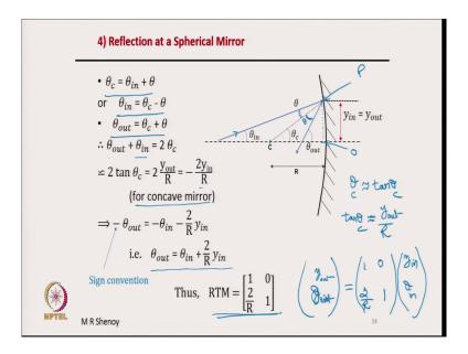
Now, let us go further reflection at a spherical mirror. So, again the geometry of the problem is shown here. So, a ray which is coming from some arbitrary ray which is incident at an angle theta in; so, theta in is the angle the ray makes when it is incident on the mirror at some point P, let us say some point P. And, after reflection the ray goes here making angle of incident is equal to angle of reflection this angle theta will be equal to the this angle theta.
