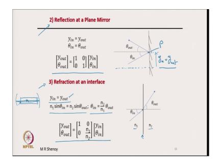
Now, let us go to the second component namely reflection at a plane mirror. So, the 1st one that we have seen is here for propagation through a distance L we are looking at propagation between mirrors. Now, let us consider reflection by a mirror. So, first plane mirror. It is illustrated here. So, this may not be the axis, axis may be here.
