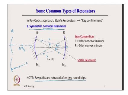
Now, some of the common types of spherical mirror resonator. So, we will follow in this ray optics approach. So, here the beam is confined means when a ray is confined to the resonator, then we call that the resonator is stable or the beam is confined to the resonator. So, this will again become clear.
