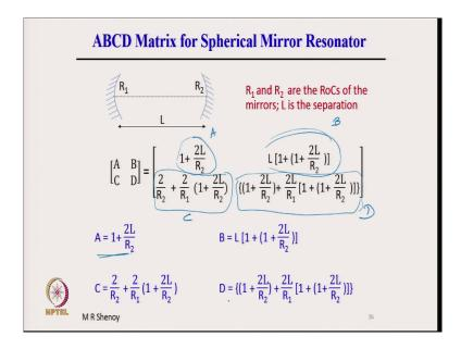
So, if we multiply this then here is the product matrix. So, this component so, this element is A. So, it is written here this is identified as A, the second element which is here is identified as B. So, that is what is written B and this is C what you have is C. So, this is C and the last element is D.
