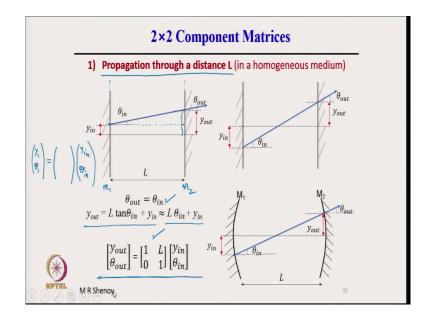
So, let us look at the 2 by 2 component matrices first propagation through a distance L. So, this is the first one, propagation through if we look back the first one is propagation through a distance L. Please see, it is not propagating through the mirror, it is from mirror M 1 to M 2, the mirror could be spherical mirror or plane mirror.
