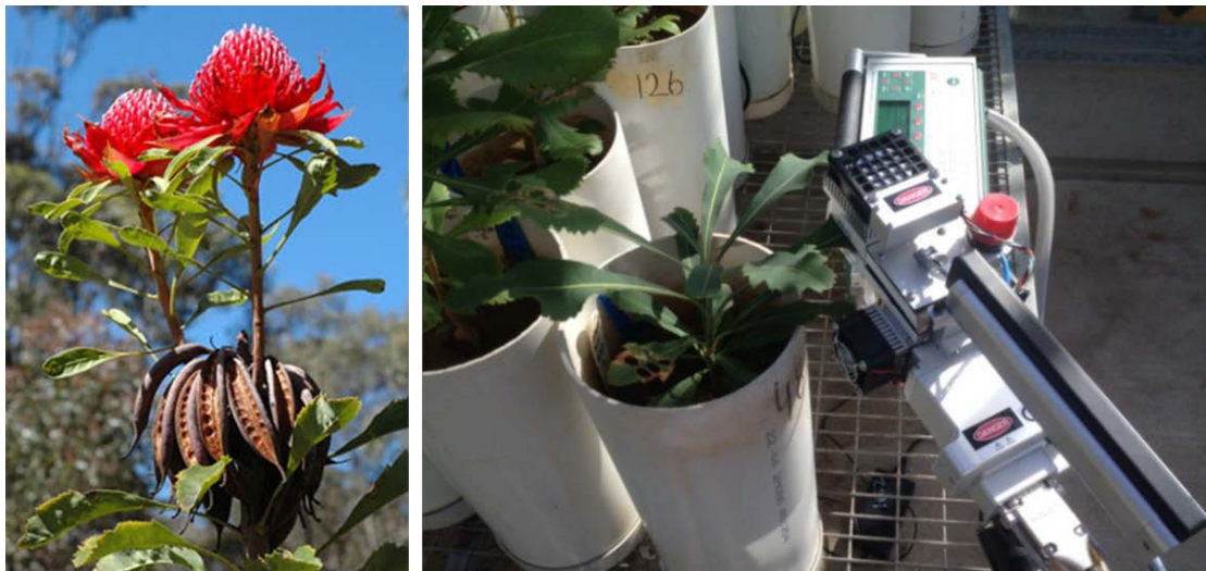
Left: Telopea speciosissima (NSW Waratah) (image from www.anbg.gov.au ); right: measuring photosynthesis and respiration of seedlings of NSW Waratah using an infra-red gas analyser (IRGA) (image from G. Huang).
