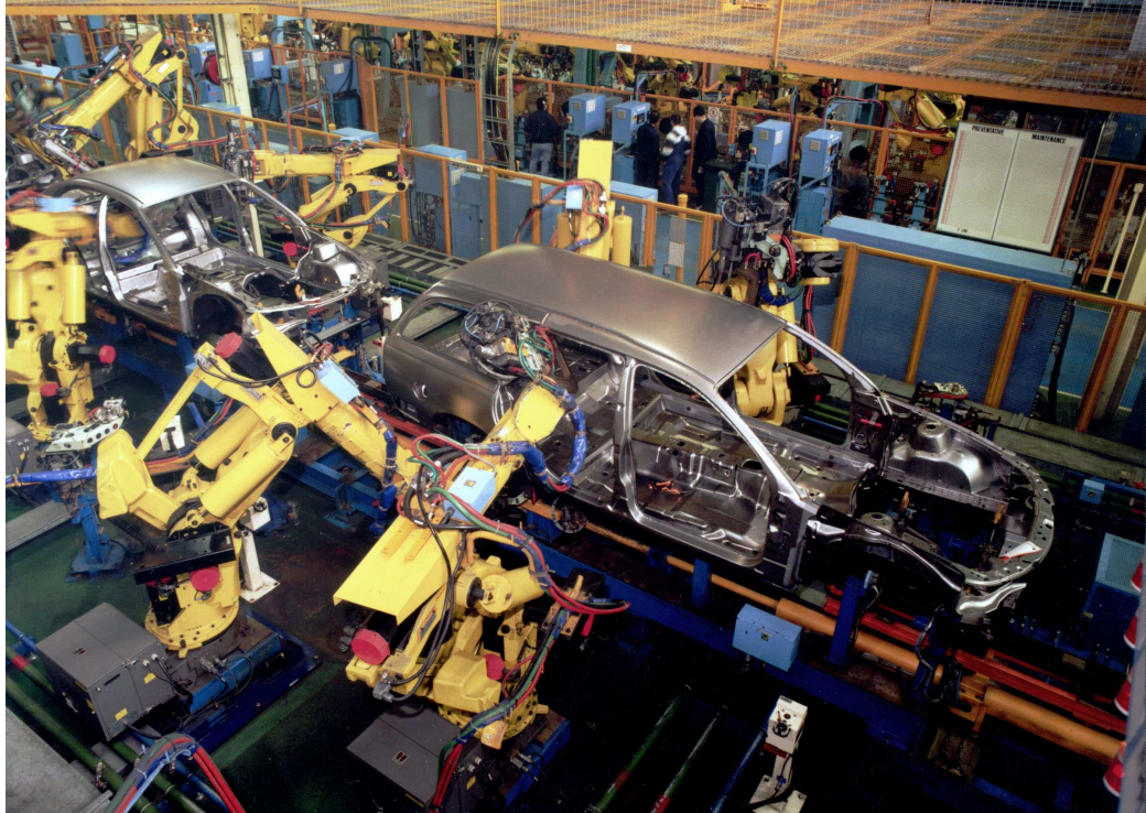
Figure 4.1: A spot-welding workcell (courtesy of General Motors).
