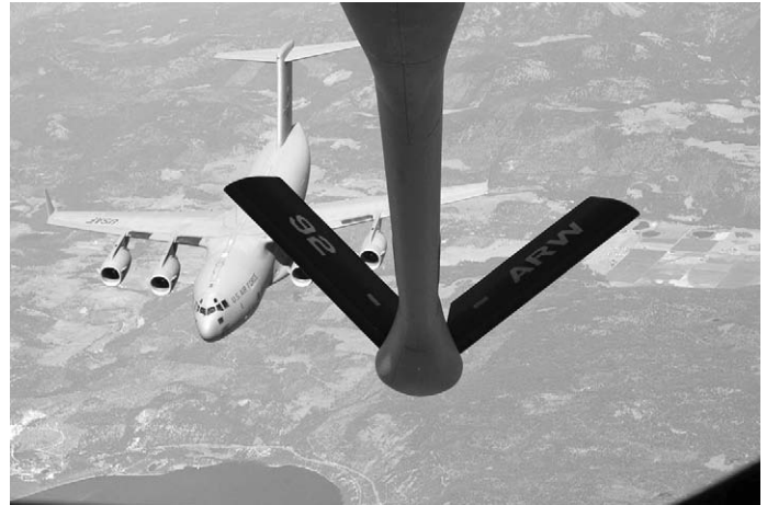
A 92nd ARW KC-135 Stratotanker prepares to refuel a C-17 Globemaster III over Moses Lake, in north-central Washington State (U.S. Air Force photo/1st Lt. Tristan Hinderliter).
