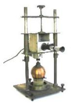
sources. It consists of a 5.5" diameter spherical chamber, the collecting electrode of which is connected to the fiber of a Lindemann-Ryerson electrometer. When viewed through the horizontally mounted microscope (projecting towards the right in the
