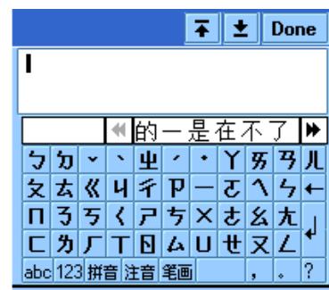
BoPoMoFo Virtual Keyboard. Includes an elements and a candidate display area.
