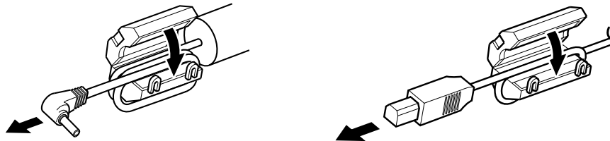
Figure 4-43: WRAPPING THE FERRITE BEADS
