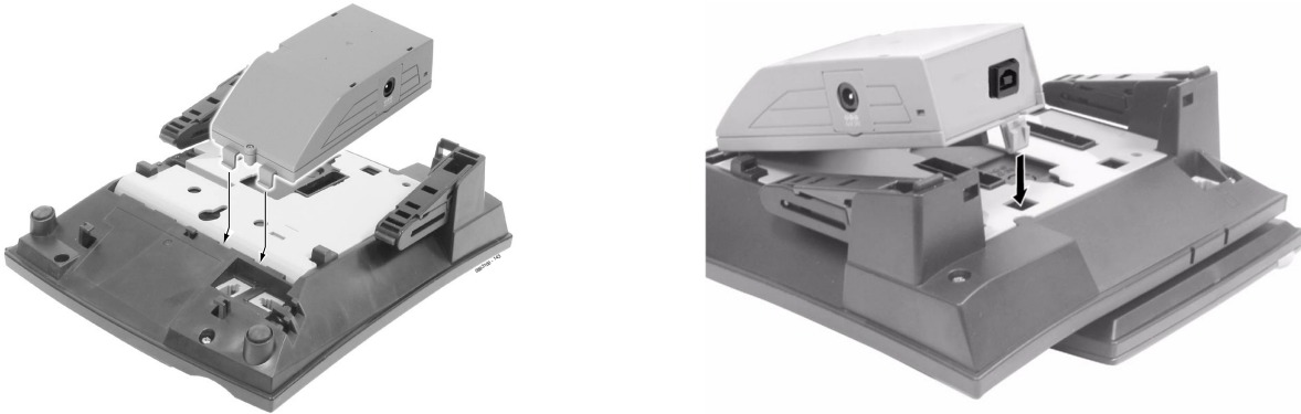
Figure 4-44: POSITIONING THE ADAPTER
