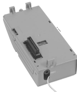
Figure 4-33: RUNNING THE CABLE TO THE ADA2
