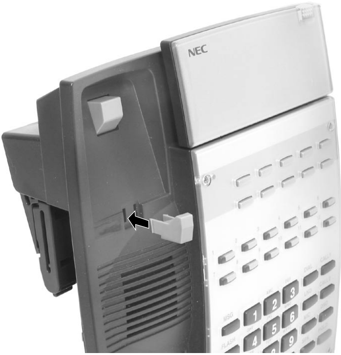
Figure 4-80: INSTALLING THE HOOKSWITCH HANGER
