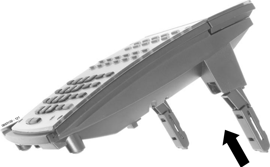
Figure 4-77: SETTING THE LEG POSITION - POSITION 3
