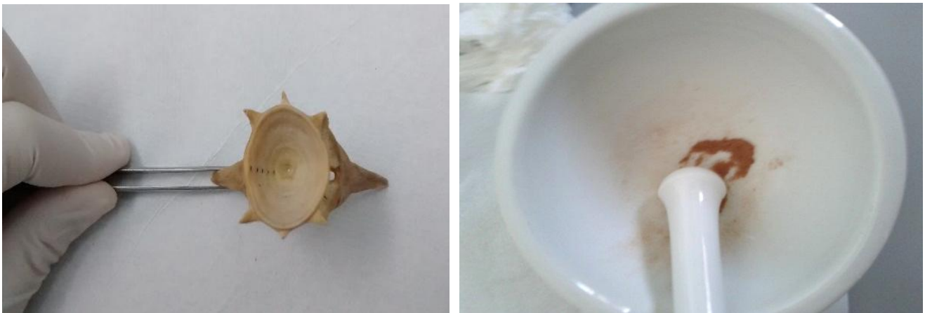
Fig. 8: A cleaned vertebra prepared for drilling and bone powder pulverized with a mortar and pestle.
