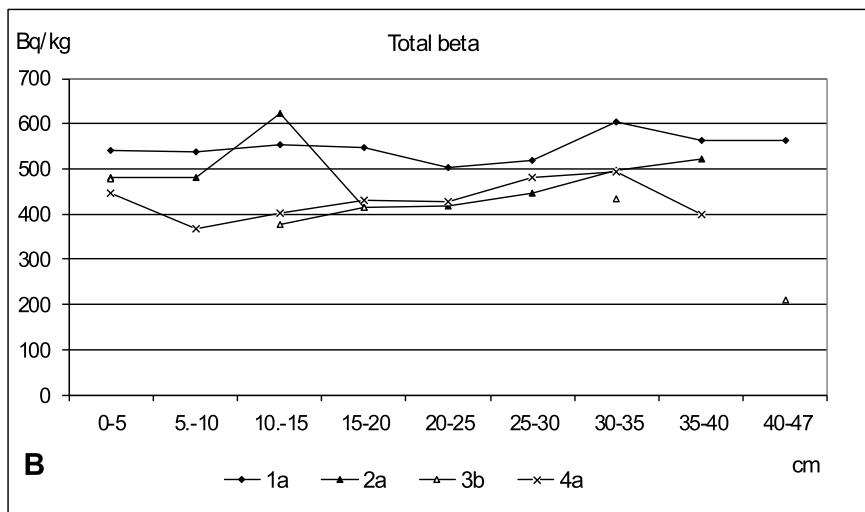
**Fig. 8.** a. Depth versus total alpha count distribution in cores; b. Depth versus total beta count distribution in cores.
