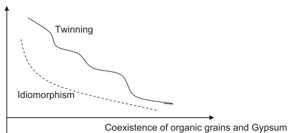
**Fig. 7.** Idiomorphism and twinning frequency of the gypsum crystals against the organic matter content.
