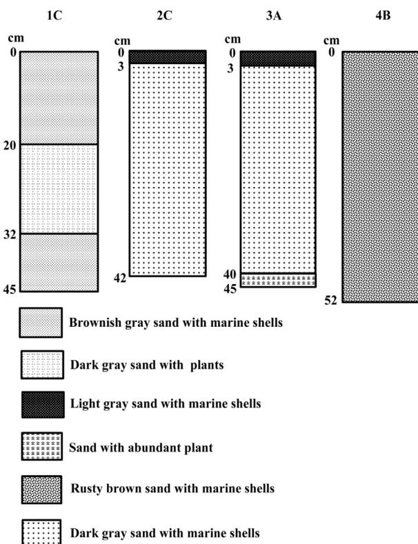
Fig. 5. Lithological identification of cores 1c, 2c, 3a and 4b.
