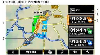
When the **MyRoutes** function is activated, up to three numbered routes are indicated on the map in different colours (orange, green, blue).
