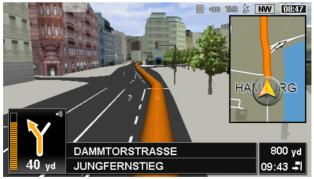
Navigation in **Real City 3D** mode takes place in similar manner to navigation in vehicle mode. The main difference is that the lane which you are to follow is not indicated in a small symbol at the right-hand edge of the screen. Instead the route shown leads directly via the correct lanes (the right-hand lane in the figure).
