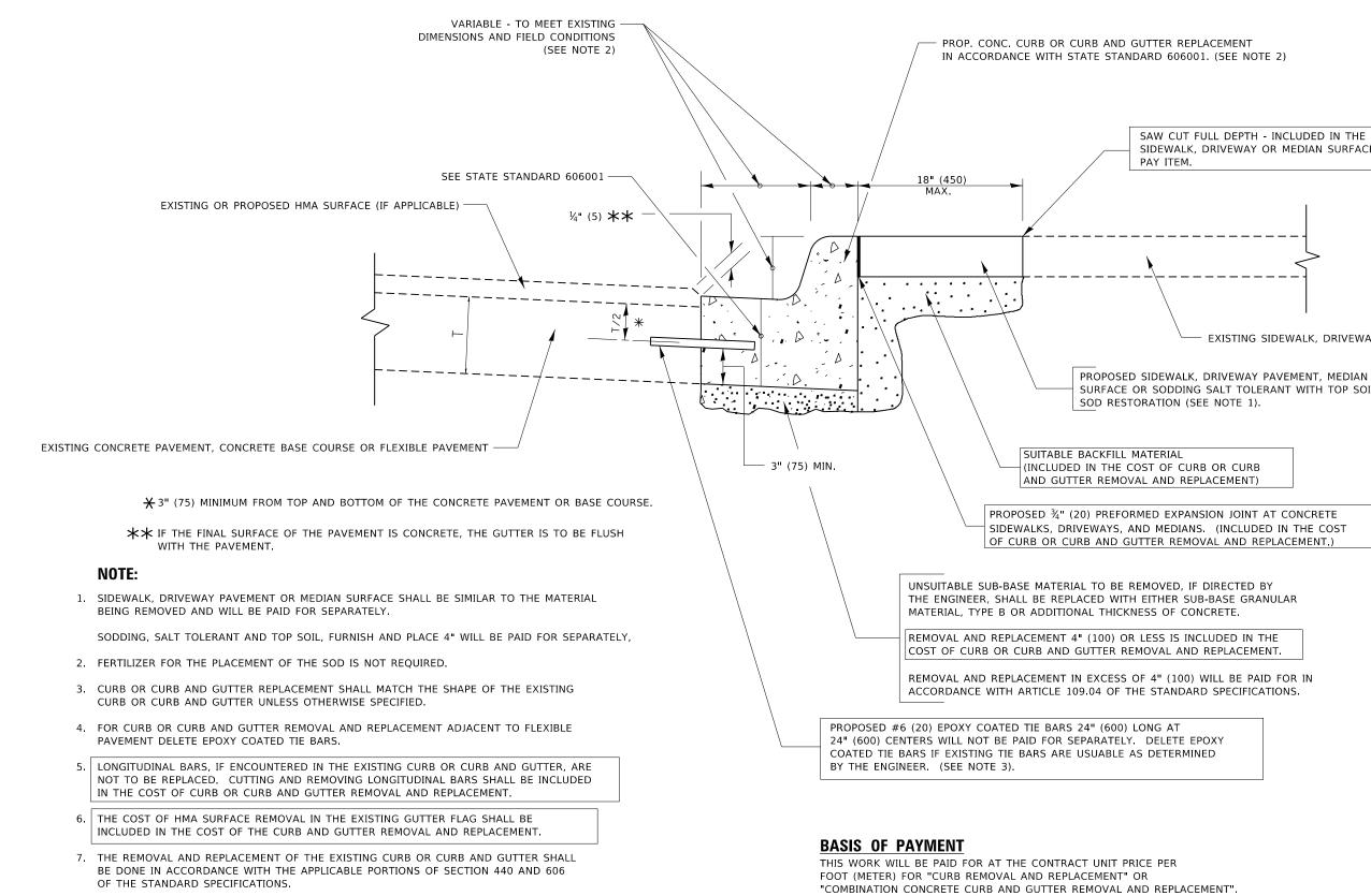
8. THE LOCATIONS OF REMOVAL AND REPLACEMENT OF EXISTING CURB OR CURB AND GUTTER SHALL BE DETERMINED BY THE RESIDENT ENGINEER AT THE TIME OF CONSTRUCTION.
