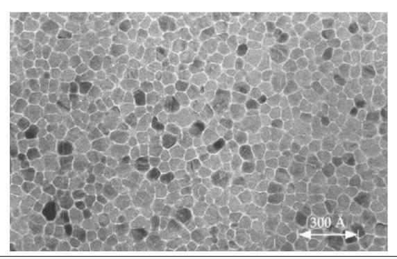
TEM micrograph of the Komag isotropic magnetic film around 1996 timeframe. White regions at the grain boundaries are filled with segregated oxide phases, containing oxides of Co, Ti, Ta, and Cr.
