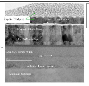
Cross-section TEM micrograph of typical PMR media used in the industry, showing various layers. (Figure 12-5)
