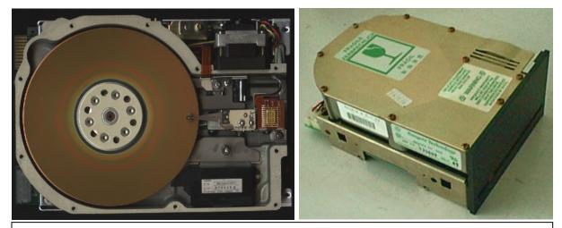
Seagate ST-506 Drive, designed to fit into 5<sup>1</sup>/<sub>4</sub>-inch floppy bay of IBM PC. Drive had 5MB capacity on 2 oxide disks. From Wikipedia (Reference 5-3).
