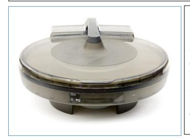
IBM 3348 Data Module for the IBM 3340 drive, containing either two or four 14-inch disks with capacities of 35 or 70 MB. The module had a spindle with bearings, head carriage, and a head-arm assembly with two low mass flying head per surface (Reference 4-1). Image courtesy of Computer History Museum.
