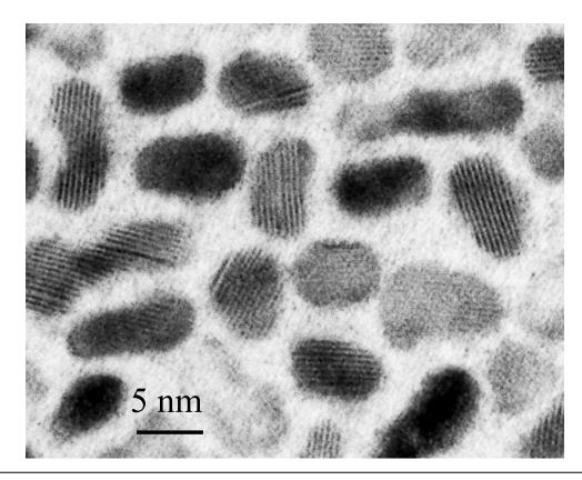
TEM micrograph of the magnetic layer for oriented longitudinal media in the 2005 time frame. The lines inside the bean shaped magnetic grains are individual atomic planes which are separated by  $\sim 2$  Å or 0.2 nm. Each of the magnetic grains is essentially a single crystal grain of Co-Pt-Cr based alloy. The white regions are amorphous material containing mostly chromium and boron which serves to isolate the magnetic grains from each other.
