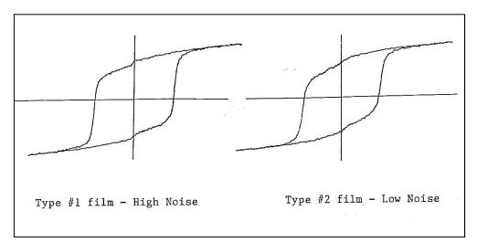
Comparison of the magnetic hysteresis loop between high noise (more square) on the left vs. low noise (less square) media on the right. The difference in hysteresis loop is quite subtle, but it is quite distinctive, and very recognizable from the micro-magnetic model that I developed at PARC.
