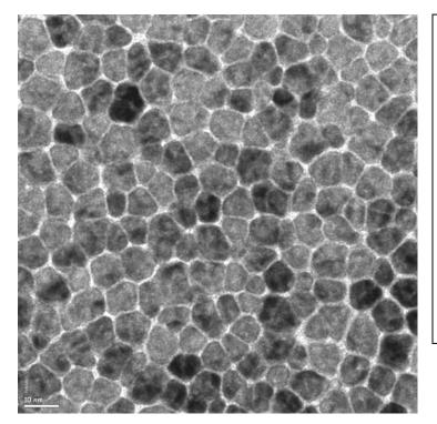
TEM micrograph of the PMR magnetic layer. Alloy consists of Co, Pt, Cr, and variety of oxides of Co, Cr, Ti. The white area between the grains is an oxide phase that separates the grains. Each grain is about 7-8 nm diameter. This type of film supports areal density of ~ 400 Gb/in<sup>2</sup> density.
