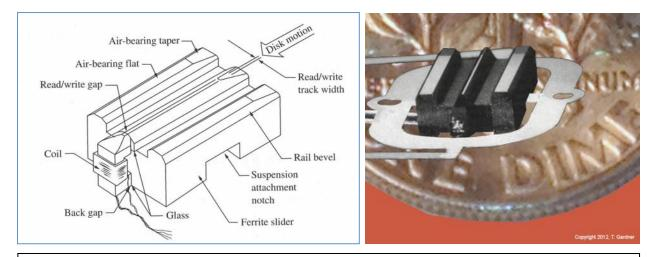
Schematic of ferrite head used in IBM 3340 drive, and photo of the head with the suspension. Dimensions: 4.0L x 3.2W x 0.86T mm. Photograph courtesy of Tom Gardner.
