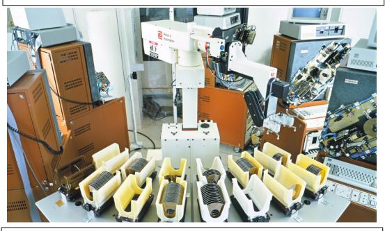
Automated disk certifier test station developed by Phase 2 Automation under the direction of Scott Chen and Steve Miura. Komag was one of the first independent media companies to develop this level of automation for disk certification. Note the IBM PC with two floppy drives which ran each ProQuip certifier.
