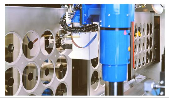
Developing automation to load/unload disks from the sputter tool was critical. Ron Allen created a team to develop internal capability for robotics from the first S1 sputter tool. The photo above is for a robot used on later sputter machines. Disks also used center plugs to cover the hole to avoid RF interference during sputtering, which are not shown.
