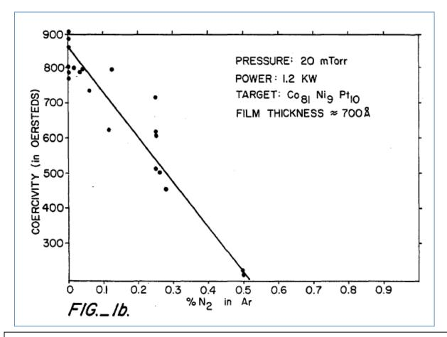
From US Patent 4,749,459 showing the effect of adding nitrogen gas during sputtering in reducing coercivity of the media.
