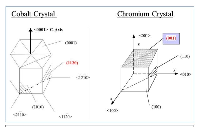
Crystallographic notation for cobalt and chromium lattice structure. In epitaxy between cobalt and chromium crystals, (001) planes in chromium would be mated with  $(11\overline{2}0)$  planes of cobalt.
