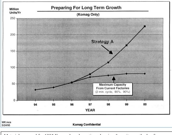
Material prepared for 1995 Komag board meeting, showing the unit growth plan for Strategy A, later renamed Plan A. "2 min. cycle and 90%, 90%" in the inset refers to the sputter system output speed, 90% product yield and 90% utilization of sputter systems which we were trying to achieve at the time.
