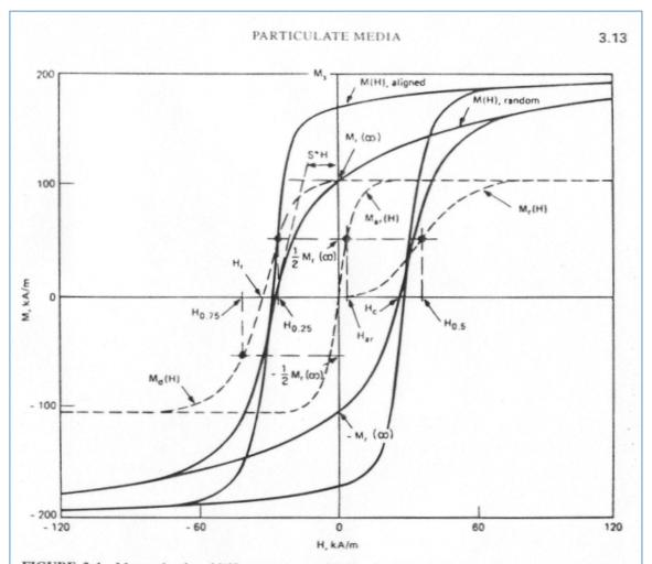
FIGURE 3.4 Magnetization M(H), remanence  $M_r(H)$ , dc demagnetizing remanence  $M_d(H)$ , and anhysteretic remanence  $M_{ar}(H)$  of a sample of randomly oriented  $\gamma$ -Fe<sub>2</sub>O<sub>3</sub> particles. For the same particles, partially aligned, M(H) is also included.
