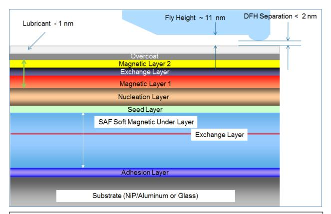
Construction of PMR media (2011) showing the complexity and the number of layers that are used. This type of construction was used for media up to around 400 Gb/in<sup>2</sup> areal density. (Figure 12-4)
