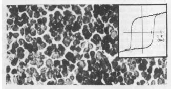
Fig. 6(b) Isolated particles, 50 µ (B-H loop insert)
