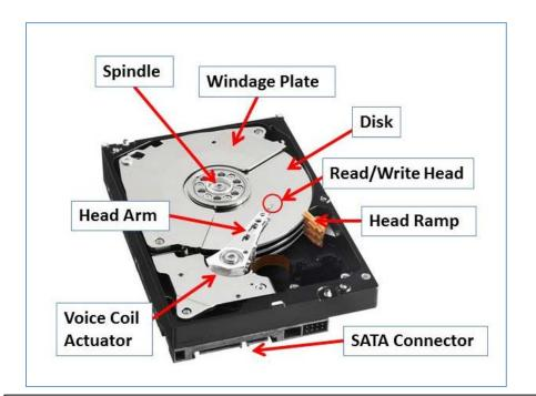
Key components in a modern disk drive. Motor is hidden inside and below the spindle. The drive is a Western Digital<sup>®</sup> desktop model with 2 TB of storage.
