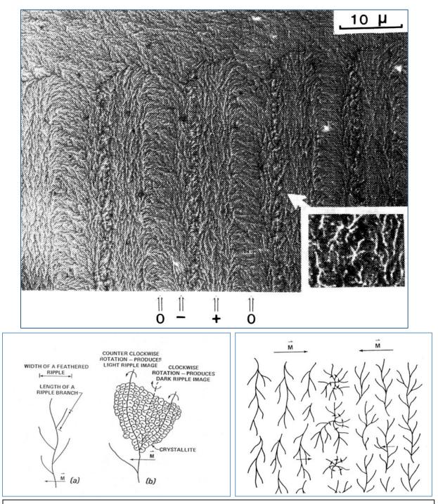
Above, from 1981 publication (Reference 4-14) showing Lorentz TEM image of recorded bits and transitions. Drawings below explain the Lorentz TEM image in terms of how it relates to the microstructure of the sputtered Co-Re grains. The Lorentz image appears as it does, because of the strong inter-particle exchange coupling between the grains. Bright star-like pattern signify strong inter-particle exchange which widens recording transitions.
