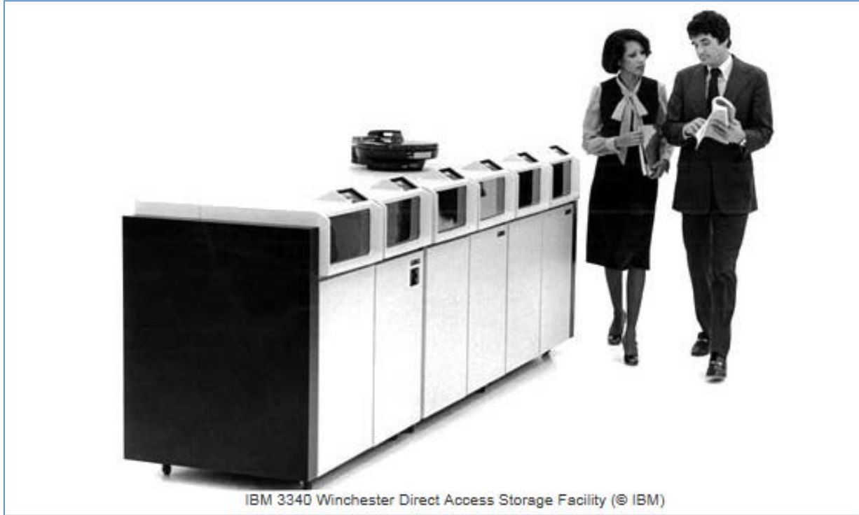
View of IBM 3340 drive, with IBM 3348 Data Module pictured on top. System was announced together with IBM 370 model 115 processor in 2, 4 or 8 unit configuration, with 280 MB total capacity with 35 MB IBM 3348 Data Module. Image courtesy of Computer History Museum.
