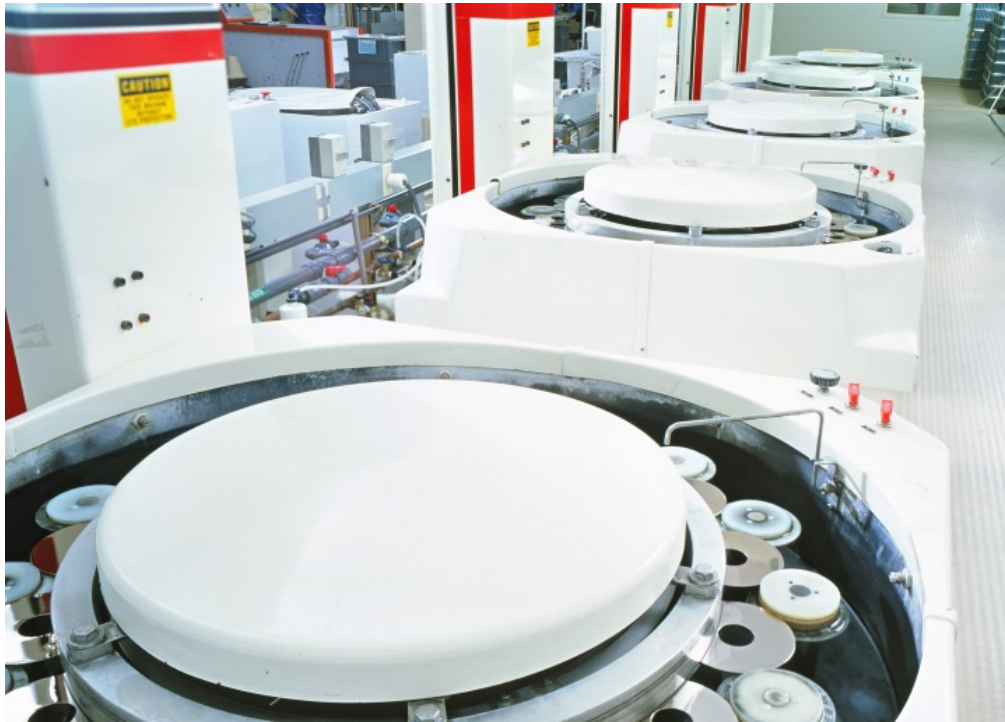
Early version of SpeedFam polishers that were used to polish and also texture the aluminum/NiP substrates. We purchased hundreds of polishers from SpeedFam and became their biggest customer for a while.
