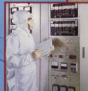
Top Left Inset: NiP plating line made by HBS Bottom Left Inset: Substrate polishing machine made by SpeedFam Corp. Main photo: S3 Sputter system in S.Hillview Drive Facility, panels loaded with 5.25-inch disks
