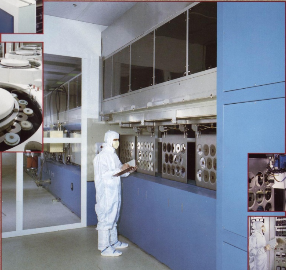
Top Left Inset: NiP plating line made by HBS Bottom Left Inset: Substrate polishing machine made by SpeedFam Corp. Main photo: S3 Sputter system in S.Hillview Drive Facility, panels loaded with 5.25-inch disks
