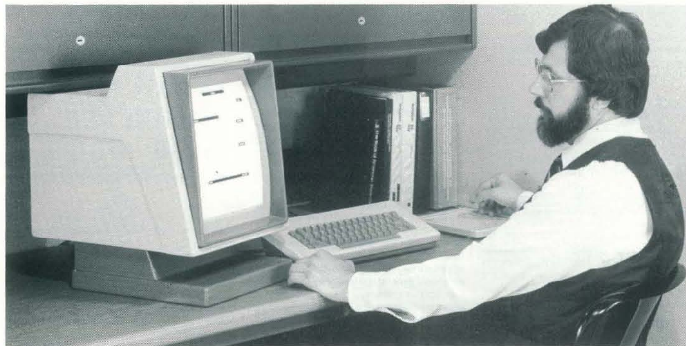
The PERQ machine provides substantial mass storage, high speed processor, a PASCAL programming environment, and a high resolution bit-mapped display.
