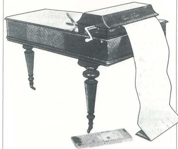
Figure 10. An example of a mechanical piano using a form of punched paper tape technology similar to the Jacquard Loom. The lever behind the playing handle controls the dynamic level.
