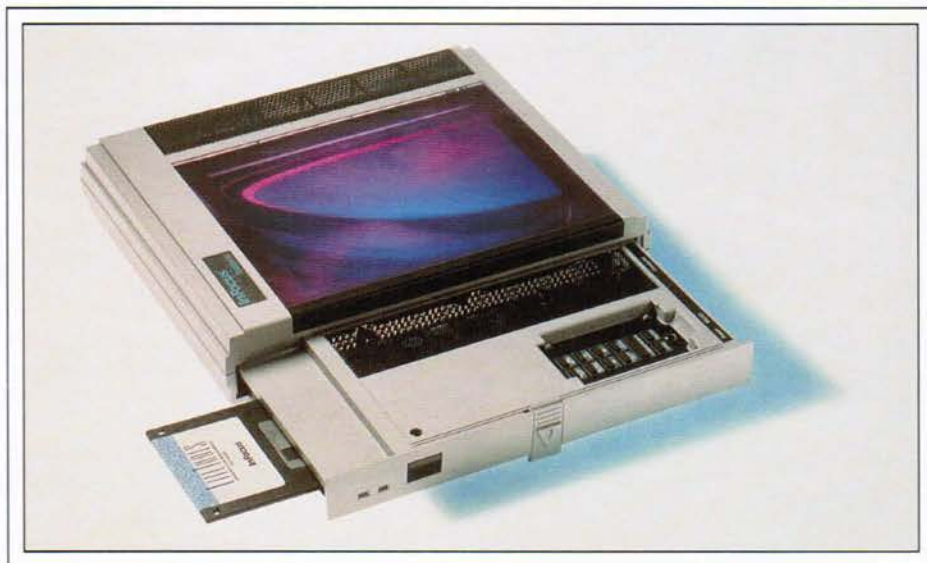
Fig. 1: This In Focus Panelbook will play a slide show from its floppy-disk drive without the need for an attached computer.
