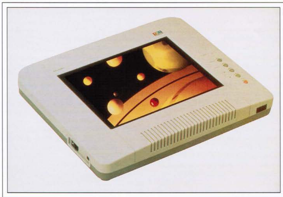
Fig. 3: Sharp's QA-1750 panel displays 16.7 million colors.
