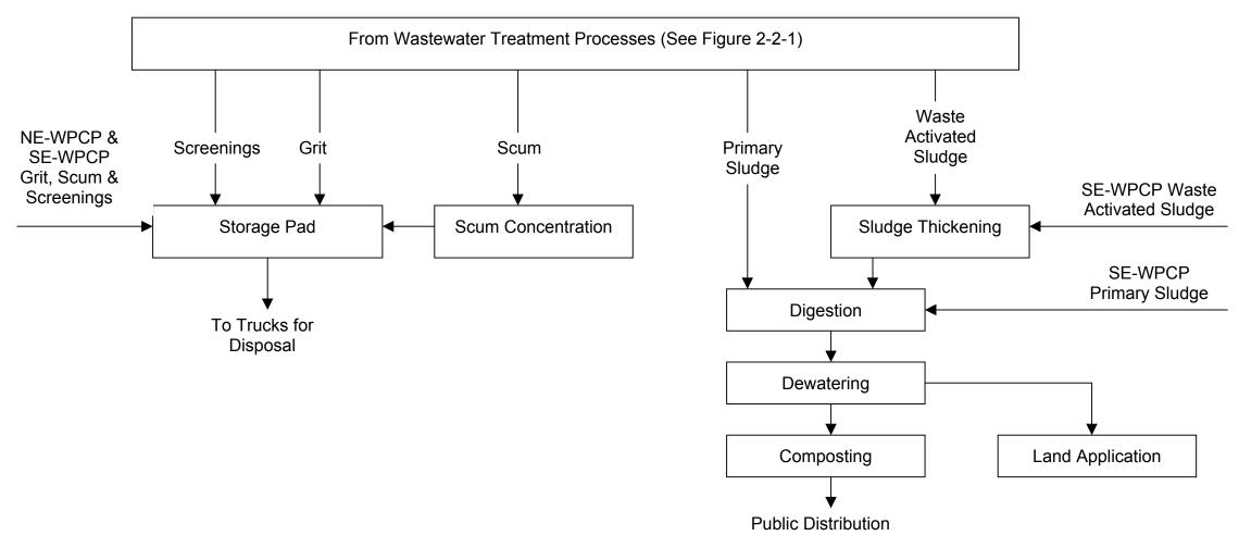
Process Plan Diagram – Sludge and Other Solids Treatment Processes
