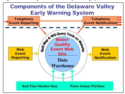
Figure I.1.2-1 Components of the Early Warning System
