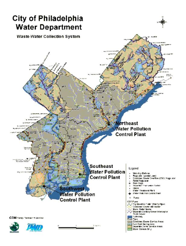
Figure 1 - PWD wastewater collection System
