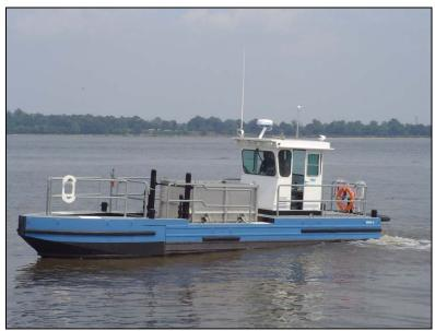
Figure II.F-3 Floatables Skimming Vessel in operation
