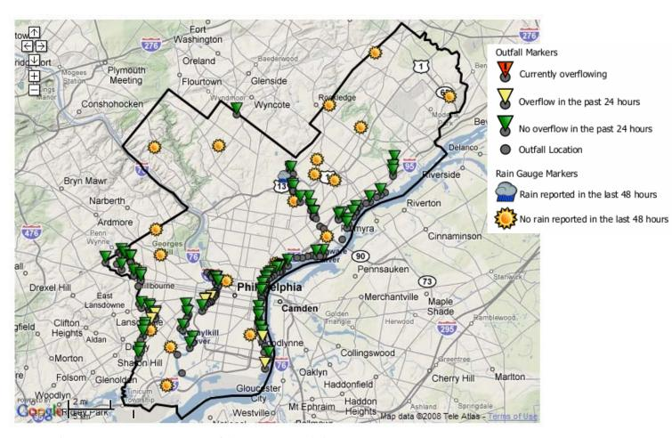
Figure II.H-2 Screen capture of the CSOcast website
