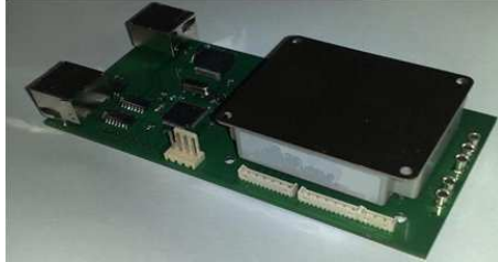
Fig. 3. ARCHIE: Brushless Motor Driver
