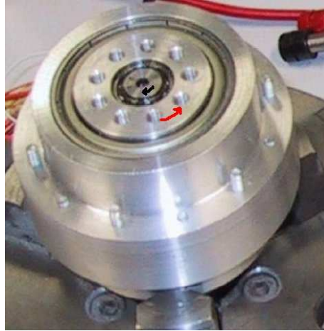
Fig. 2. ARCHIE: Modular Joint Design combining a brushless motor and a harmonic gearbox
