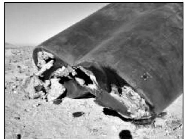
Burned water tank
