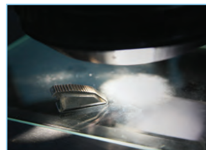
Shadowgraph wedge inspection
