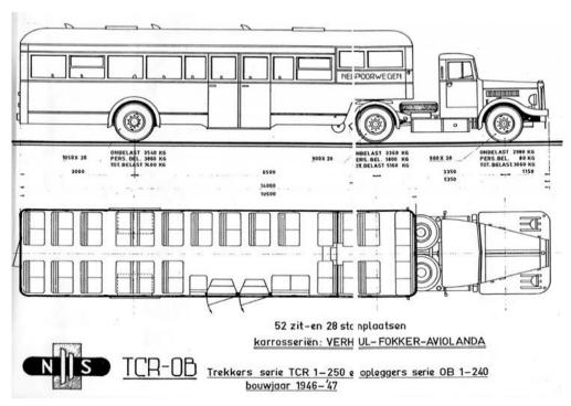
Figure 3" Blue-print for transport vehicles used by the Dutch Railways (©Frans Gommers, eindhoven-in-beeld.nl).
