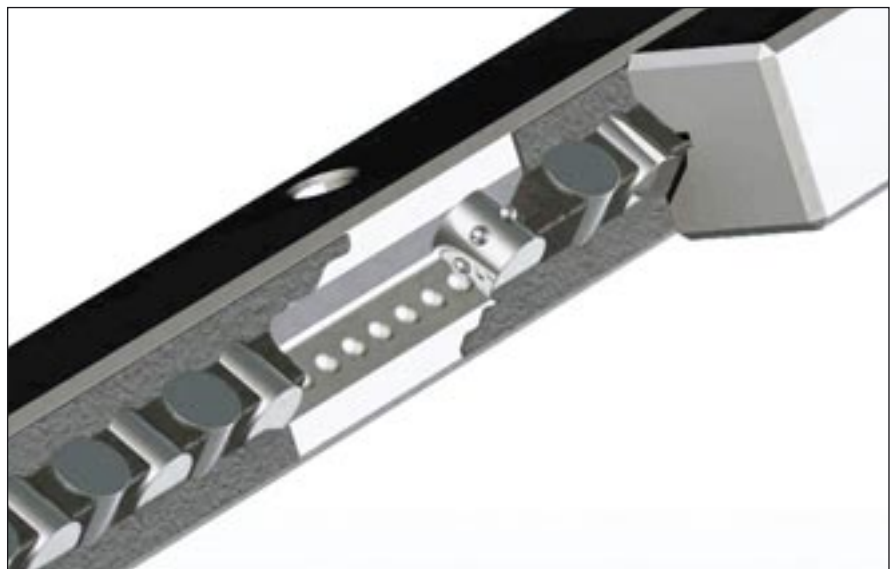
Cage creep is prevented by the studs that roll into the raceways' depressions.
