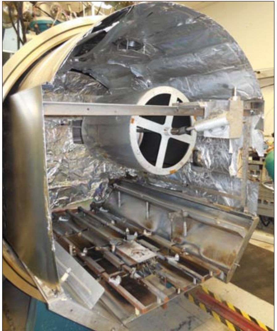
Materials are evaporated onto spaceflight hardware, blanket material, or other surfaces that require exterior passive thermal control.
