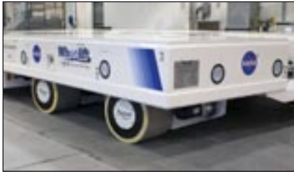
Motion control for the Wheelift wheels is handled by Beckhoff AX5000 servo drives and AM3000 servomotors.
