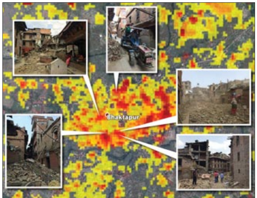
Photos of the damage in Bhaktapur, Nepal, are overlaid on a damage proxy map derived from COSMO-SkyMed satellite data. Colors show increasingly significant change in terrain/building properties (including surface roughness and soil moisture). Red is most severe. (Image Credit: NASA/JPL-Caltech/Google/DigitalGlobe/CNES/Astrium/Amy MacDonald/Thornton Tomasetti)
