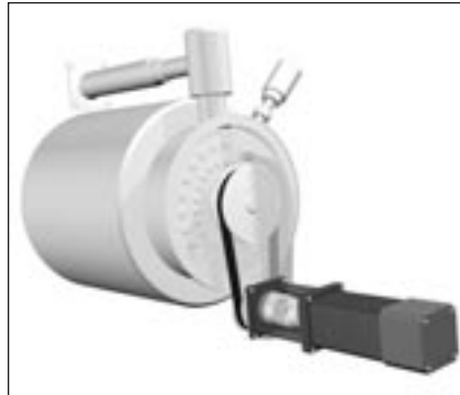
Mechanically advantaged mechanism by a belt and planetary gearhead.
