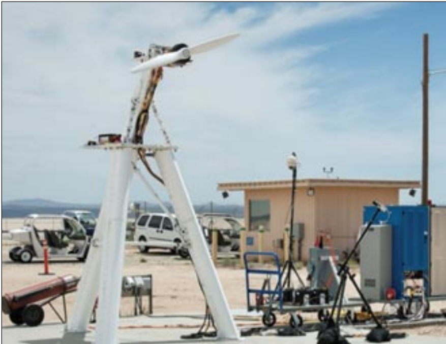
NASA Armstrong's modular stand for testing aircraft electric propulsion systems with propeller installed.
