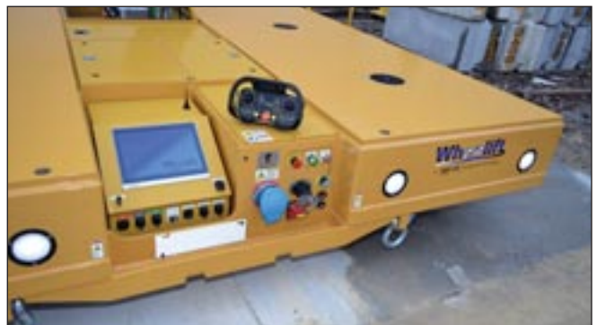
A PC-based control platform from Beckhoff Automation ensures that the Wheelift can handle changing, frequently uneven terrain, and reposition SPMTs as needed.
