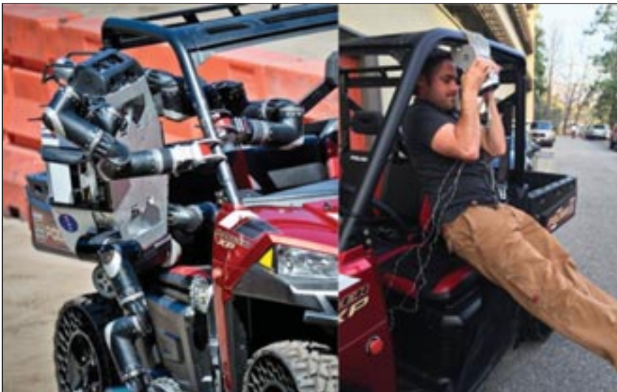
Figure 2. In its current design form, the Cam Hand is extremely strong and robust. It easily supports the 125kg mass of an entire RoboSimian. Its self-contained mechanism and electronics could be adapted to human anchoring devices or prosthetics.
