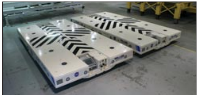
Since January 2014, Wheelift Self-Propelled Modular Transporters (SPMTs) have been used by NASA to transport SLS rockets and components from site to site.
