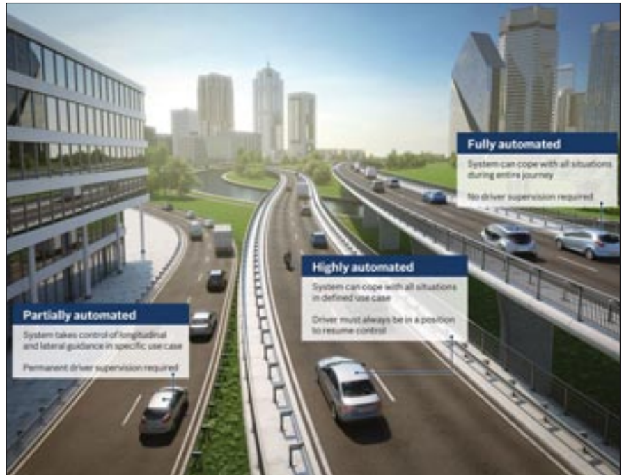
Figure 4. Automated driving will be implemented in stages. (Image Credit: Robert Bosch GmbH)
