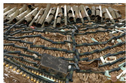
A number of 1.25lb M112 Demolition Charges, consisting of a C-4 compound, sit atop degraded weaponry scheduled for destruction
