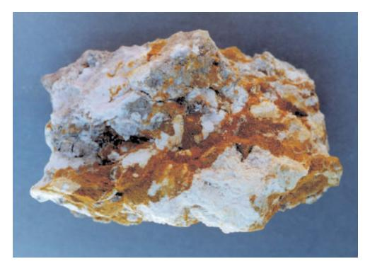
Figure 10. Hand sample, 7 x 9 cm, showing golden metavoltine vein in fine-grained coquimbite.
