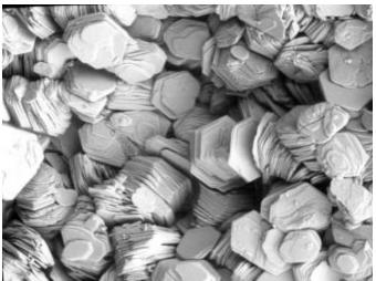
Figure 12. SEM photo of metavoltine crystals to 50 microns showing the stacked hexagonal plates.
