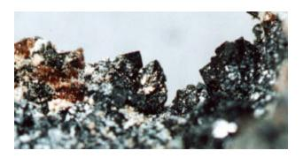
Figure 19. Voltaite specimen showing 2 mm cubic crystal outline (center top) associated with brown römerite (left).
