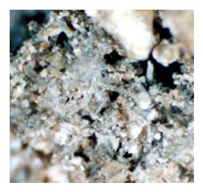
Figure 14. Typical surface showing clear to light pink, jack-straw crystals of quenstedtite. Width 4 mm.
