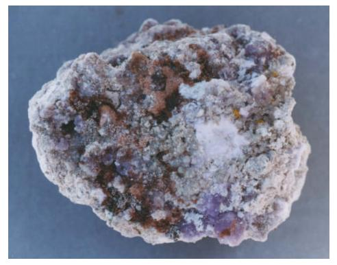
Figure 2. Hand sample, 5 x 7 cm, from the transition zone showing typical sulfate assemblage (purple coquimbite, brown römerite, gray-green krausite, and sugary-white coquimbite).
