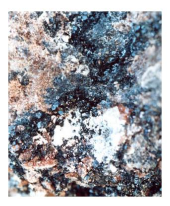
Figure 18. Typical specimen of voltaite showing black cubic outline associated with brown römerite and halotrichite. Width 1 cm.
