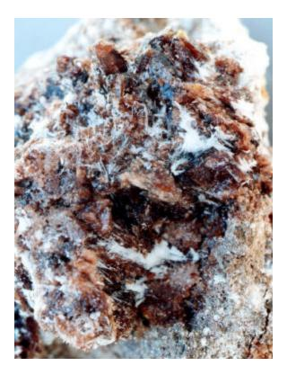
Figure 17. Typical sample, 2 x 5 cm, of dark brown römerite with white fibrous halotrichite.
