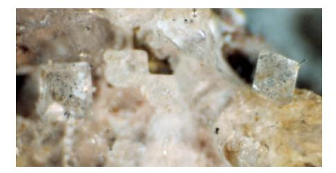
Figure 13. Clear octahedrons of potassium alum. Field of view 4 mm.
