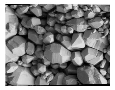
Figure 6. SEM photo of sugary-white coquimbite showing the bipyramidal habit of the individual crystals. 10 – 100 microns.
