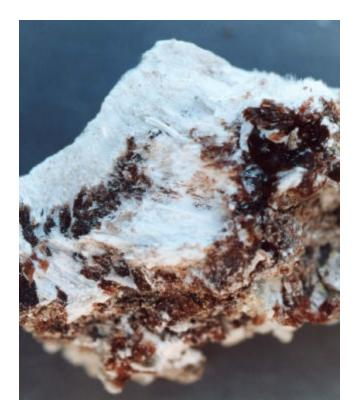
Figure 16. Sample of dark brown römerite associated with white fibrous halotrichite. Width 3 cm.
