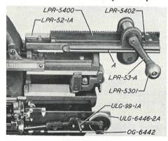
FIGURE 6 View of Plate Roller for Dupligraph Plates
