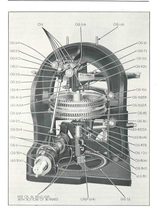
FIGURE 9 Rear View of Model 6280 Graphotype
