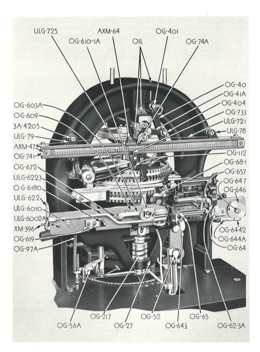
FIGURE 5 Front View of Model 6280 Graphotype
