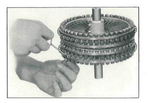
FIGURE 8 Replacing Punch
