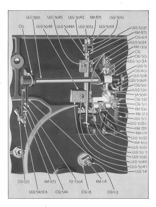
FIGURE 10 Bottom View of Model 6280 Graphotype
