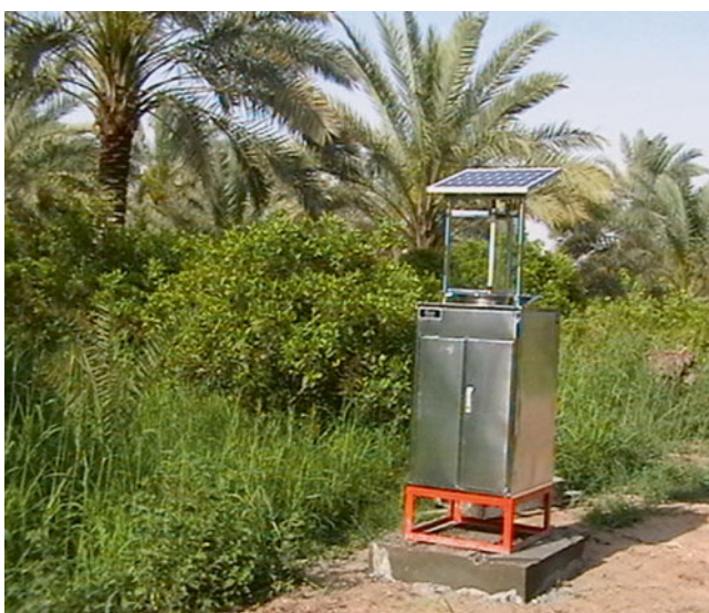
Fig. 5.22 Solar light trap (Magna Trap with lamp of 320–420 nm wavelength, Russell IPM Limited, UK) used for monitoring and controlling Oryctes spp. in date palm orchards in Iraq (Photo: Mohammed Z. Khalaf)
