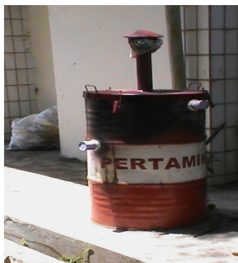
Fig. 1. Equipment for charring: actual (left) and schematic of a pyrolysis reactor (right).
