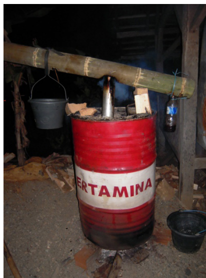
Fig. 1. A modified drum kiln with major parts—drum, cover, smoke chimney, and bamboo cooling device.
