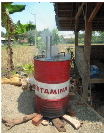
Fig. 1. A modified drum kiln with major parts—drum, cover, smoke chimney, and bamboo cooling device.
