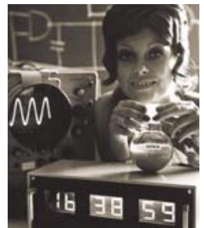
Invention of the twisted nematic cell (TN cell, James Ferguson, Martin Schadt and Werner Helfrich) – used here in a digital clock with "liquid digits" constructed by Merck in 1972.
