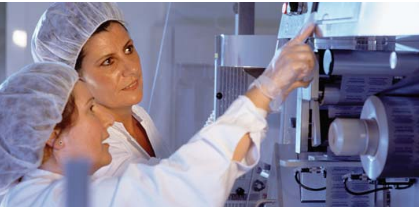
Mollet del Vallès | Spain _____ Regina Manzanera and Lidia Prades work in drug manufacture. They are checking a plant for packaging tablets in blister packs.
