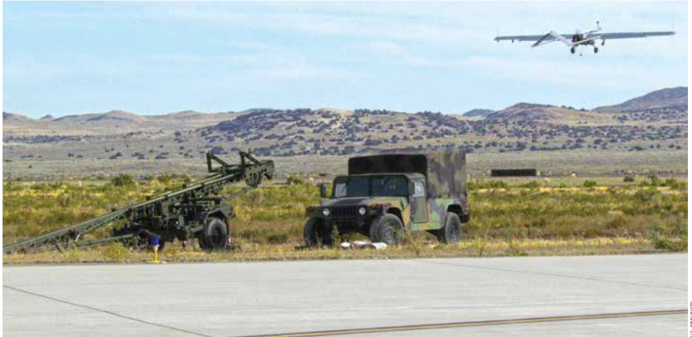
An RQ-7 Shadow Unmanned Aircraft System launches at Dugway Proving Ground, Utah.
