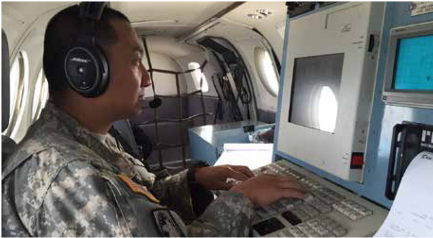
SFC Clifford Linnell checking alignments on the Automatic Flight Inspection System (AFIS) computer before flight check operations.
