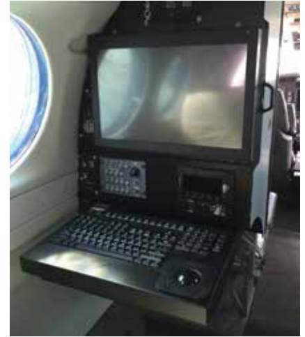
NextGen AFIS mission specialist panel in C-12S at Cairns AAF, Fort Rucker, AL 6 Jul 2016
