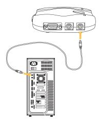
Repeat Steps 3 through 5 for each additional computer to be connected to the Switch, connecting them to the corresponding CPU ports on the side.
