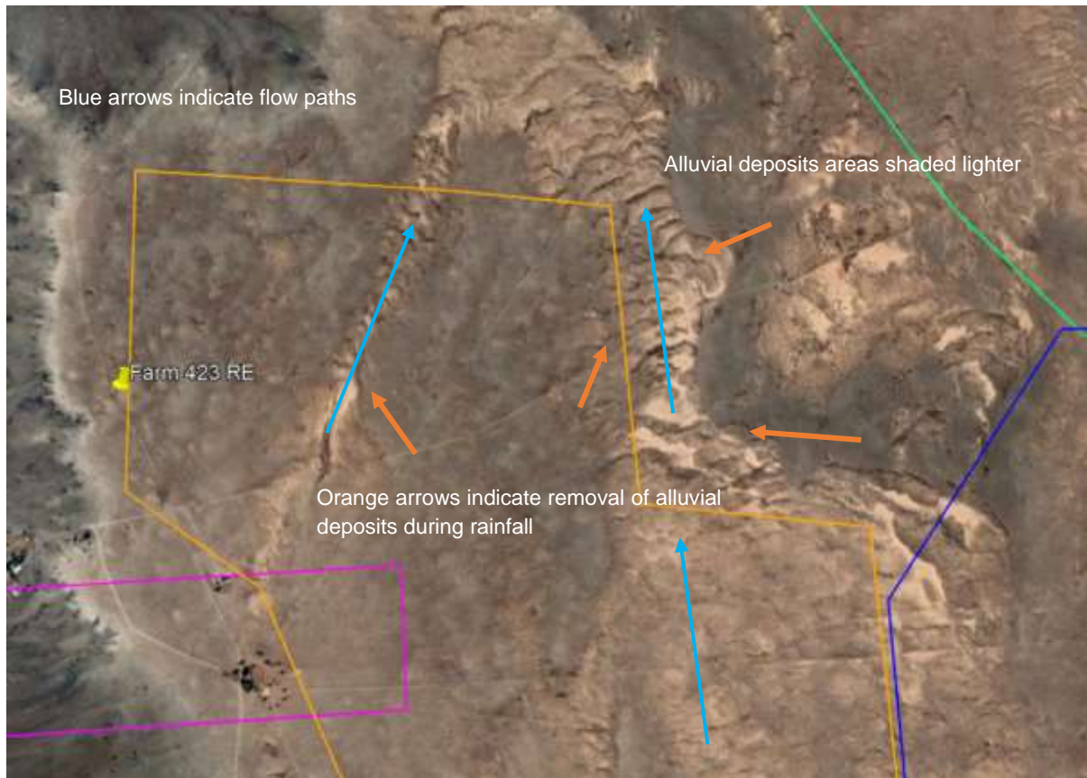
Figure 6-20: Illustration of alluvial deposits (within the Salsola PV area)
