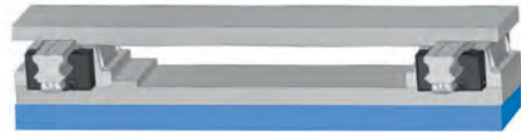
(2) Assembly of the back side of block, rail transfer
