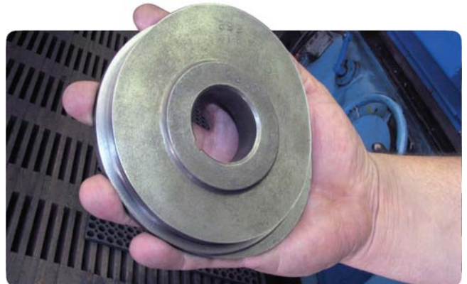
The Master Cam is a solid piece of tool steel.
