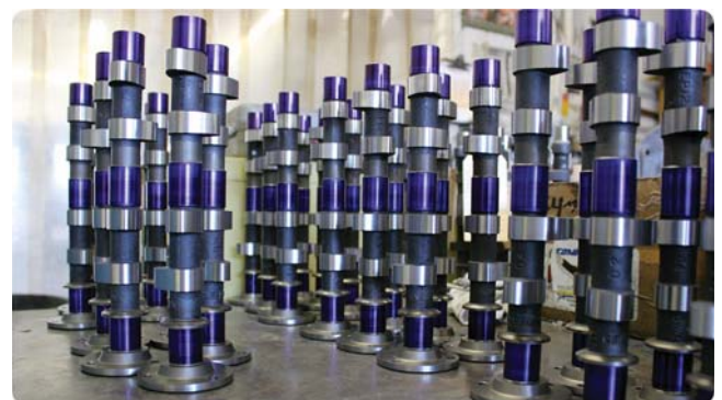
A non-metallic thermal coating is applied to every Eagle Camshaft.
