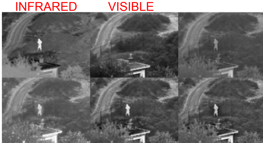
Fig. 1 Top: input IR image (left), input visible image (middle) and fused image using averaging (right); Bottom: fused image using ratio pyramid (left), LT (middle) and DT-CWT (right)
